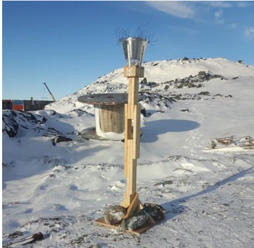
Figure 2. Dustfall sampling stand at the Meliadine site.
