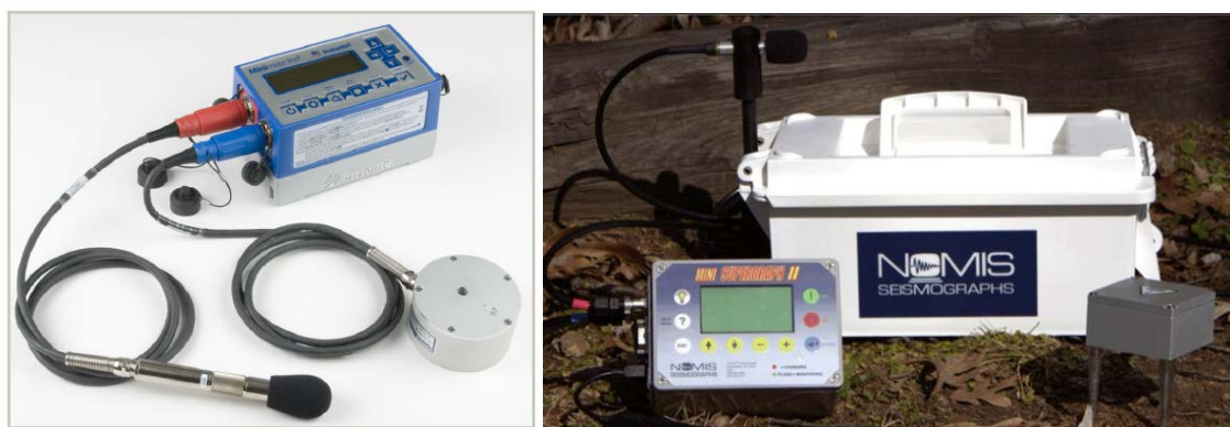
Figure 3-1 Minimate Pro4 components and NOMIS Super Graph II
