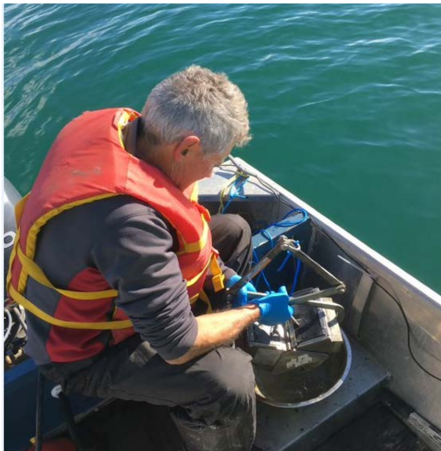
Figure 4: Sediment sampling using Petite Ponar grab
