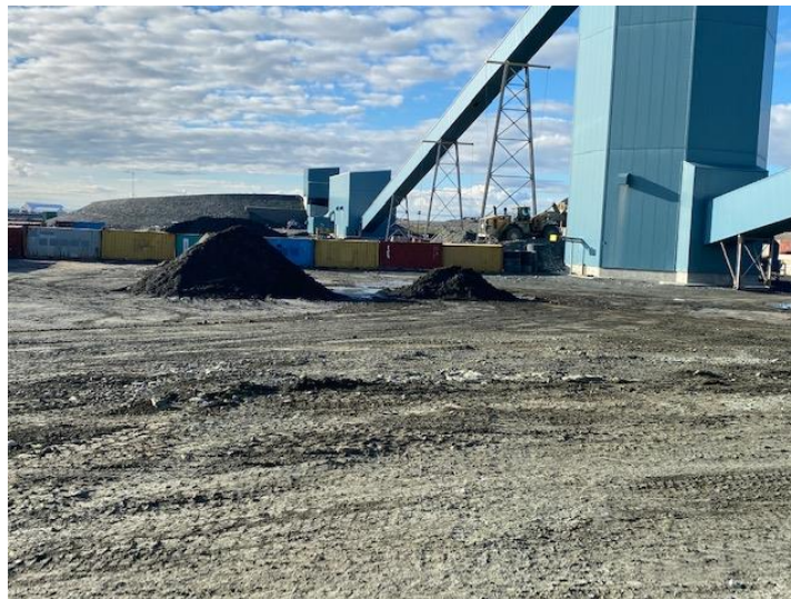
Figure 3: Spilled slurry added to existing ore feed pile for immediate reprocessing.
