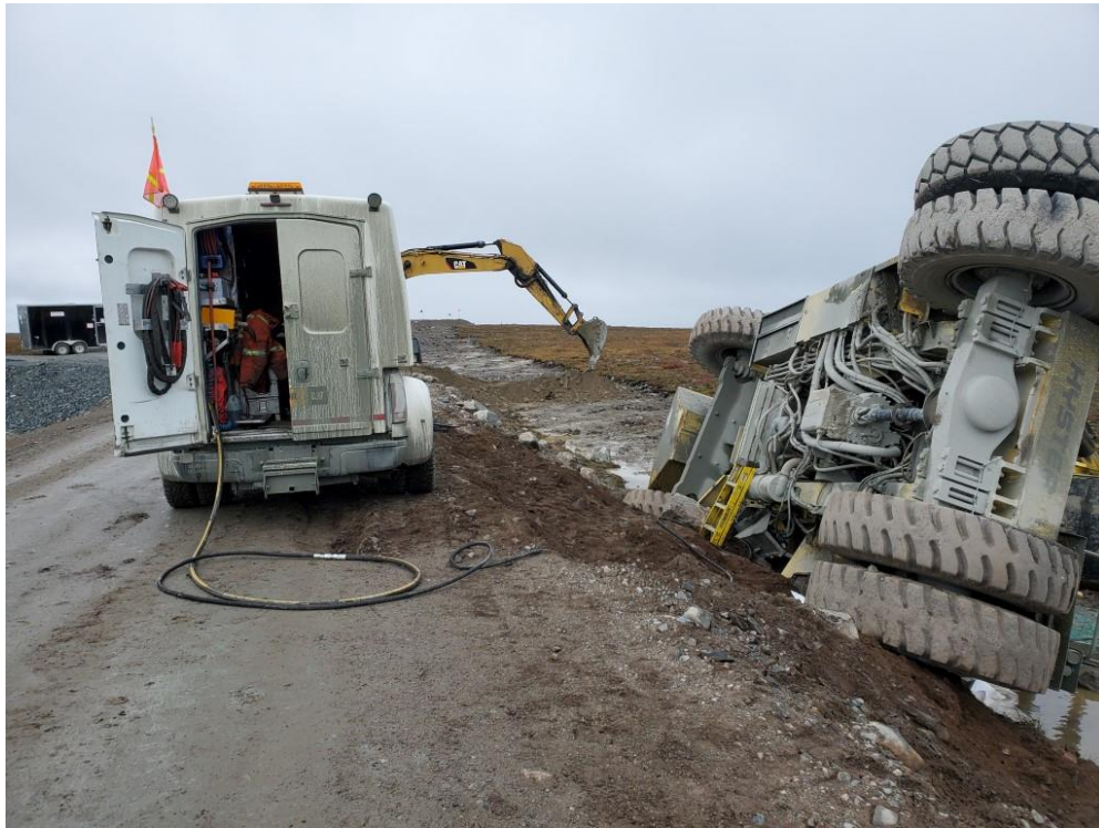
Figure 2: Upstream berm being placed while mechanic drains hydraulic, fuel and transmission systems.
