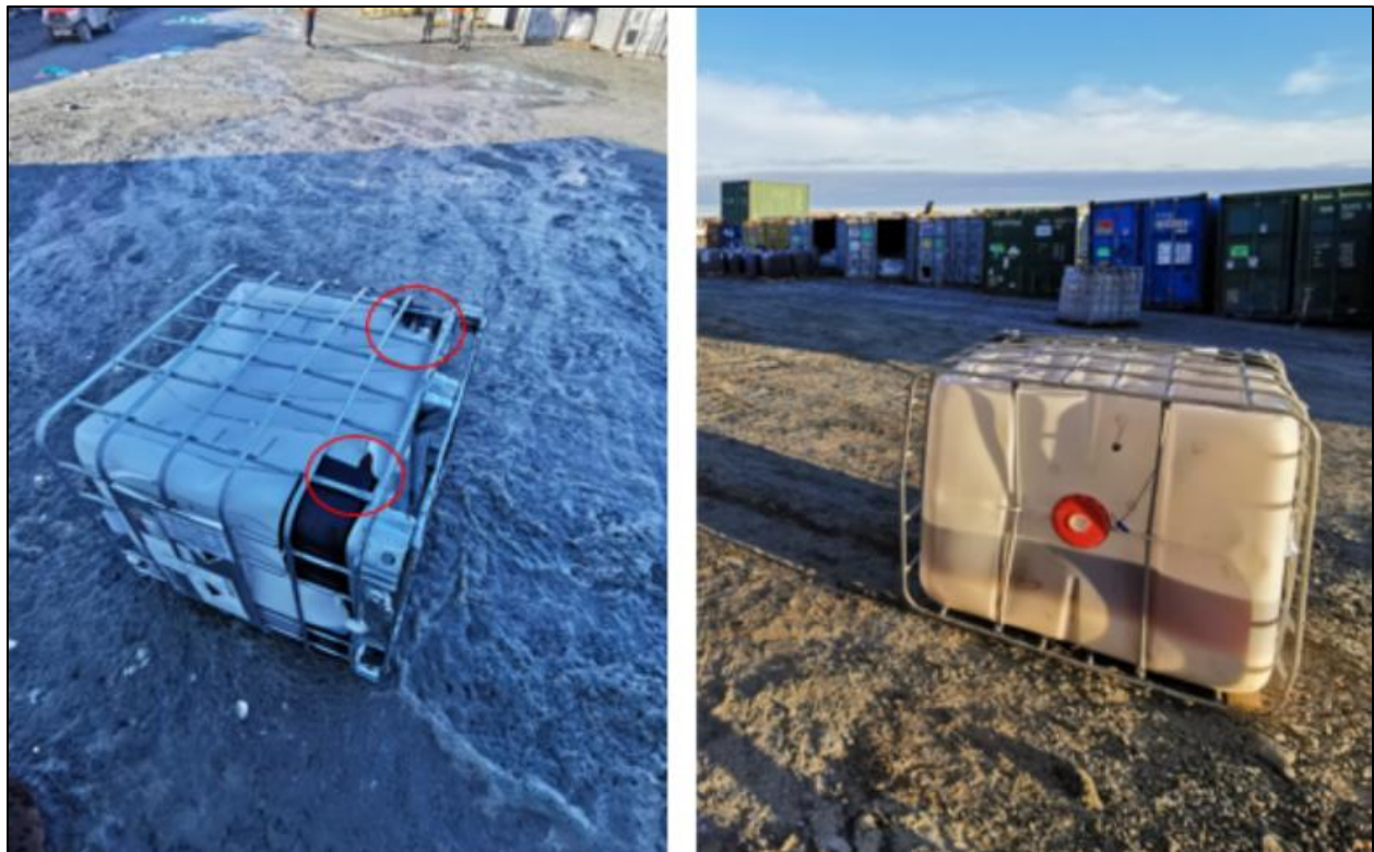
Figure 1: Punctured tote with remaining liquid inside.
