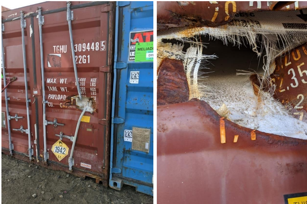
Figure 2: Damaged seacan containing Ammonium Nitrate.
