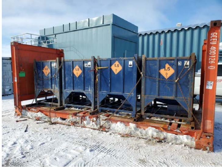
Figure 6: Steel dividers installed to improve visibility during pre-loading inspection.
