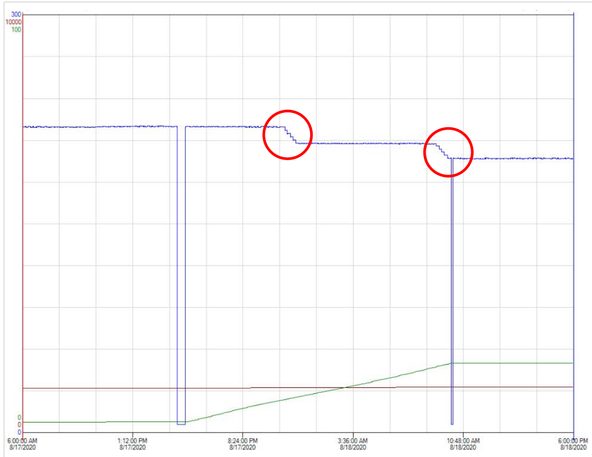
Figure 2: Main Camp Complex Fuel Tank Level (blue), CCBM Energy Totalizer (green) and CCEG Totalizer (red)
