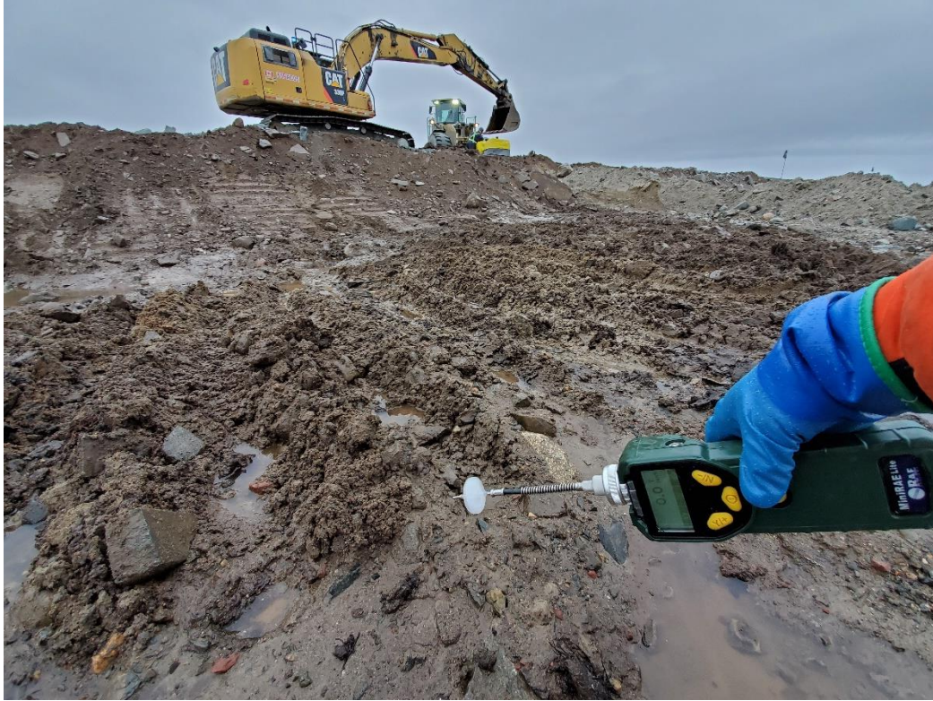
Figure 4: Mini RAE VOC detector used to ensure all affected soil was removed.
