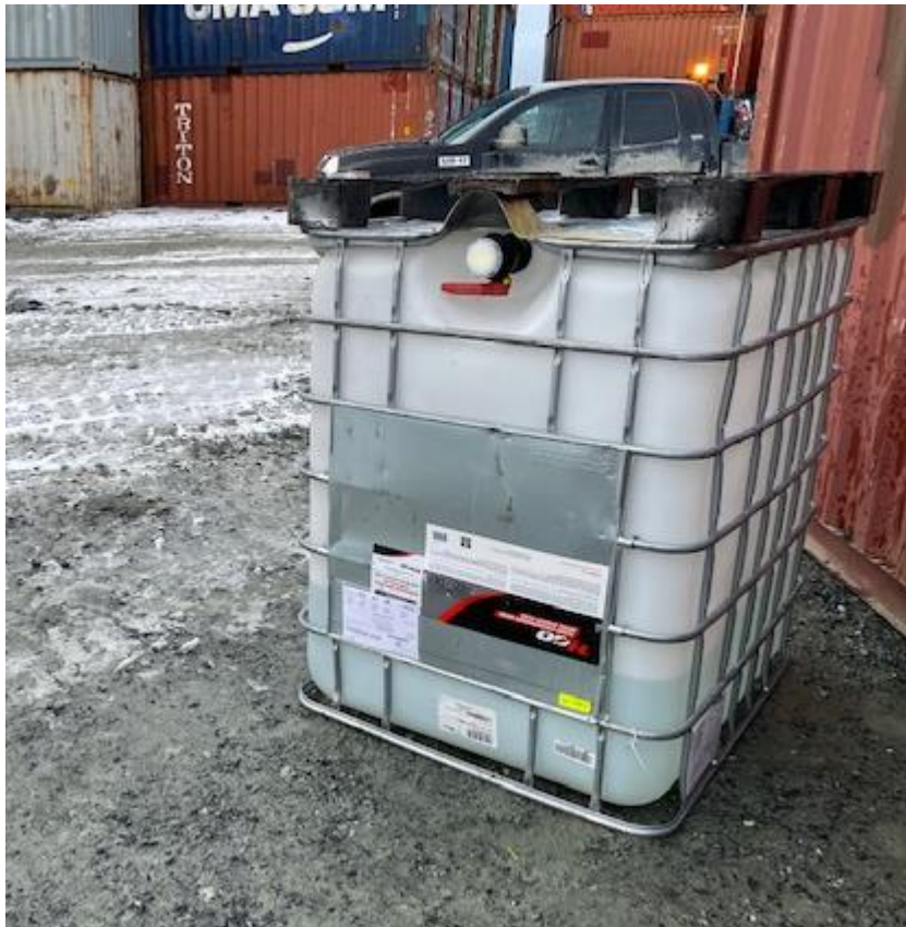
Figure 2: Tote Flipped to Reduce Volume of Urea Released
