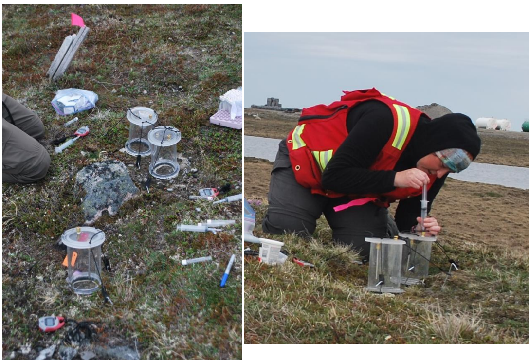
Figure 17. Static vented gas flux chambers on BSCs at drilling wastes from 1997/1998. Gas flux was sampled every 15 minutes over a 1 hour period to determine in-situ \text{CO}_2 , \text{N}_2\text{O} and \text{CH}_4 .
