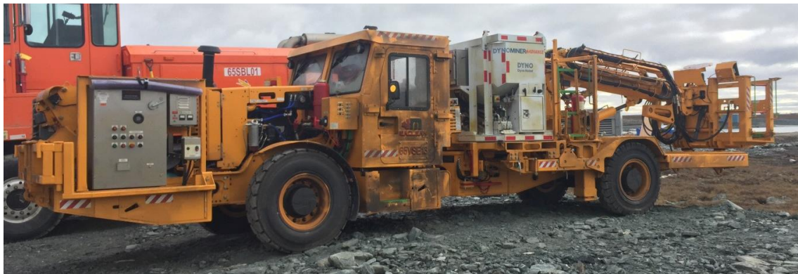
Figure 3-3 Underground Emulsion Charger – Dyno Loader
