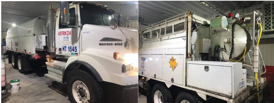
Figure 3-1 Mobile modular Emulsion Plant and Explosive Truck
