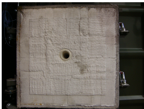
Secondary Door (refractory lined)
