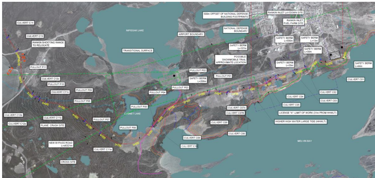
Figure 3: Bypass Road and Culvert Location
