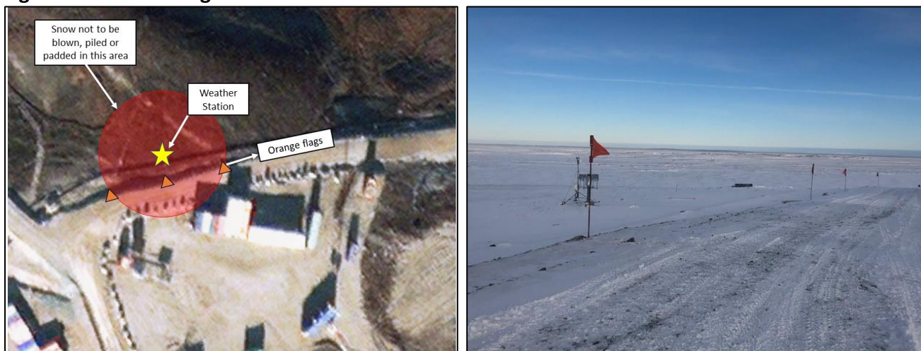
Figure 3: Snow Management around the Weather Station
