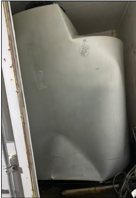
Photo 2: Sewage tank failure
