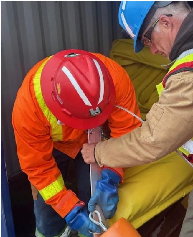
Photo 3: Demonstration to the team on how to properly connect the marine booms.
