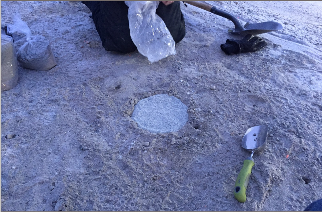
Photo 37: Modified sand cone test on final lift of Type C material on upstream fillet at Station 0+560
