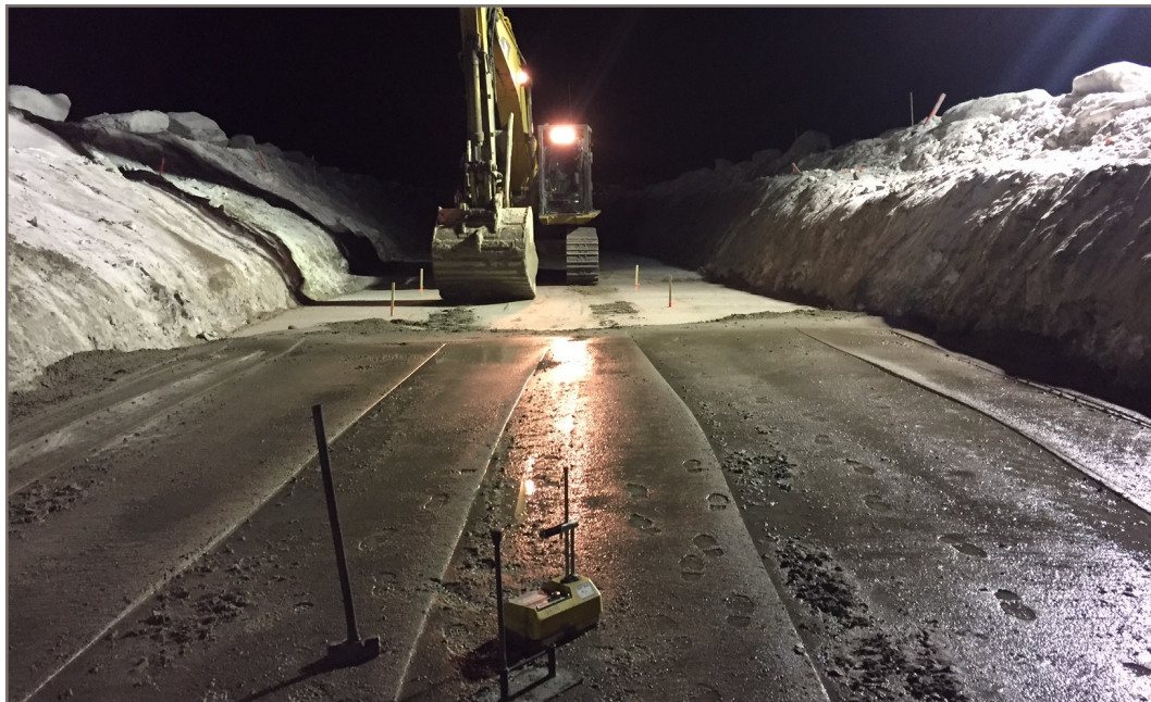
Photo 41: Compaction test on a lift of Type K material placed between Station 0+200 and 0+310
