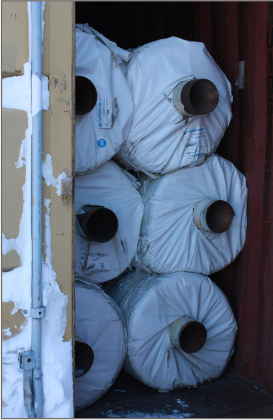
Photo 52: Coletanche ES3 liner panels in a shipping/storage sea can
