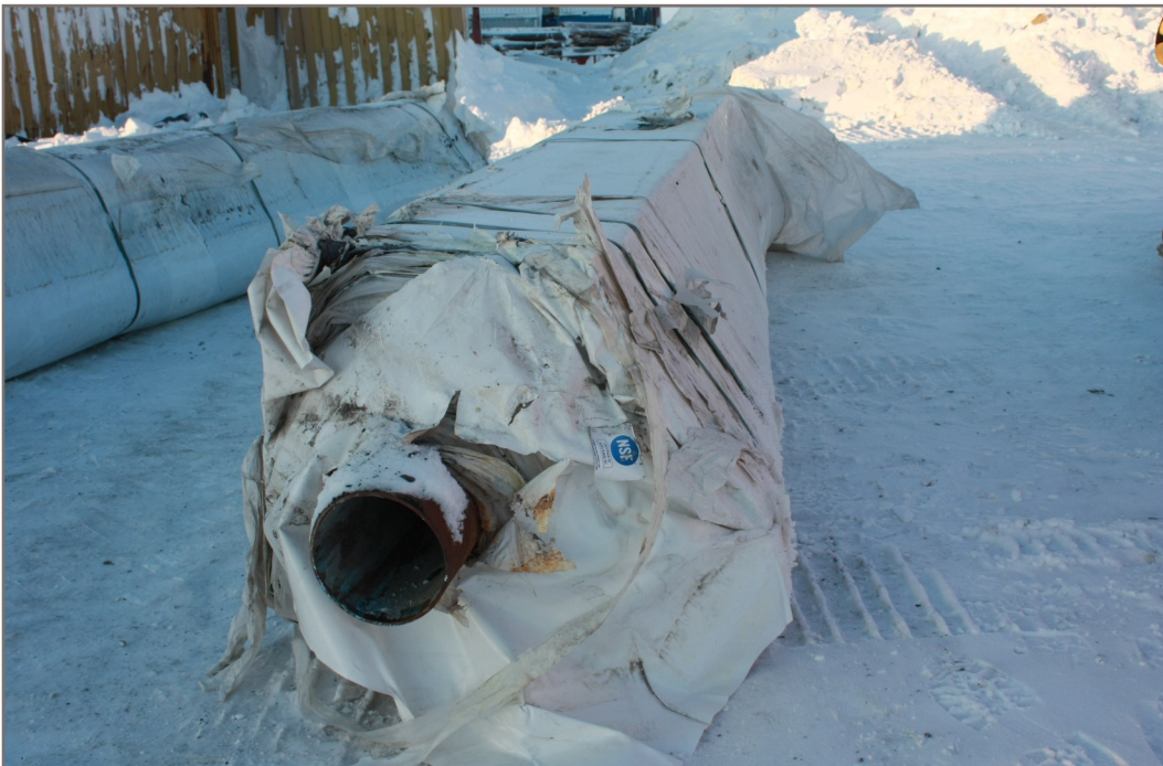
Photo 53: Deformed Coletanche ES3 liner panel pulled out of shipping/storage sea can
