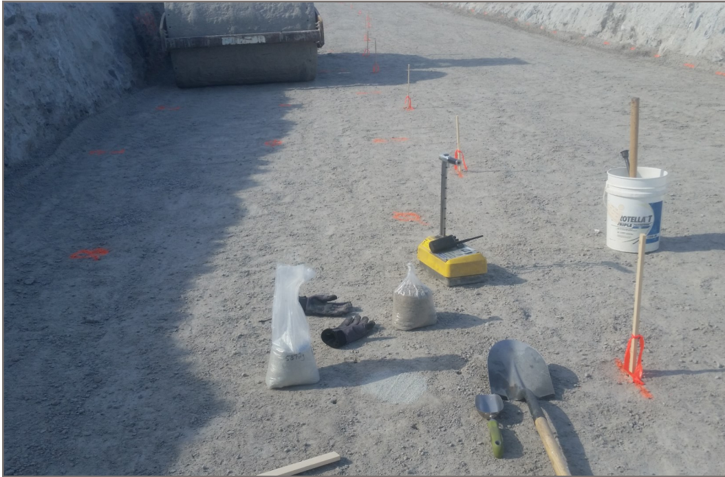
Photo 33: Densometer and Sand Cone Tests on Type F material around Station 0+260
