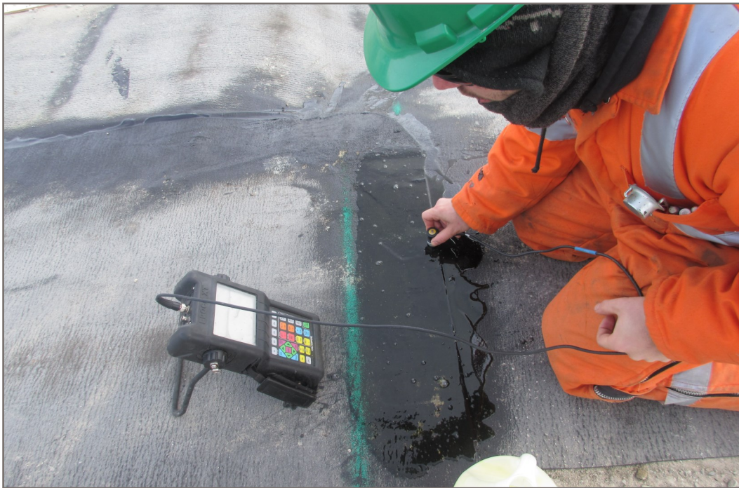
Photo 38: Performing an ultra-sonic test on a seam between two liner panels.
