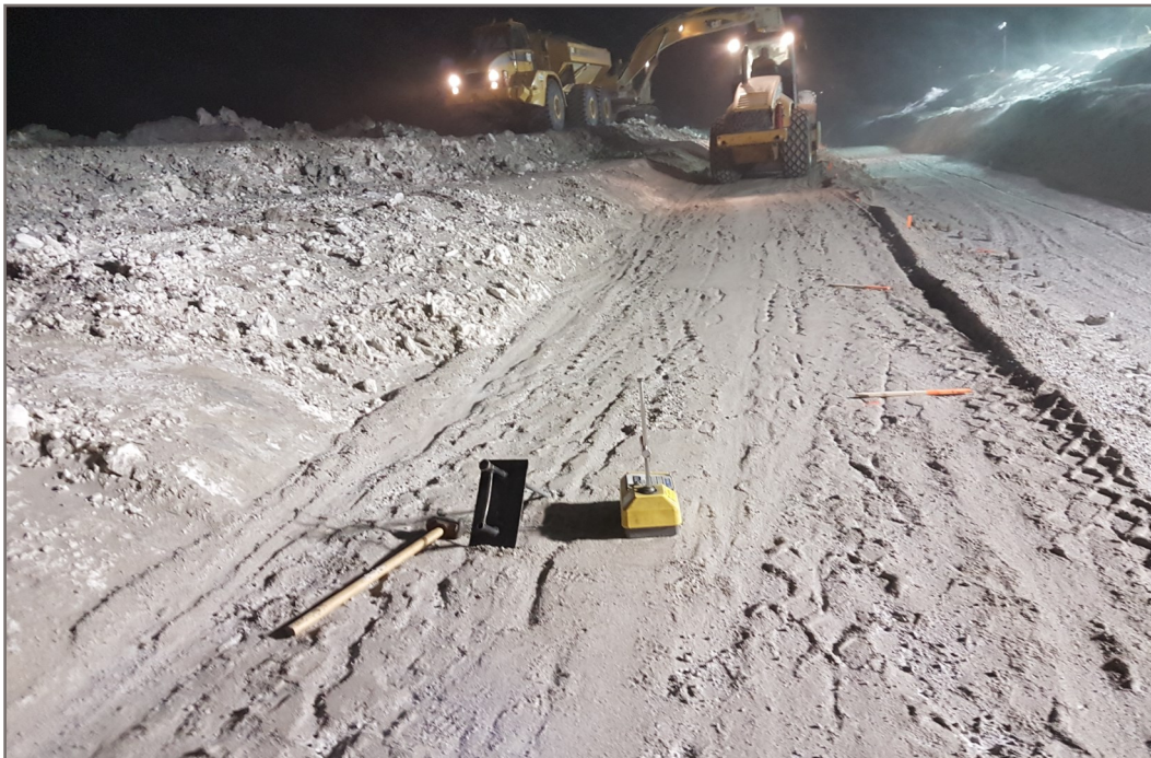
Photo 30: Densometer test on a lift of Type C fillet material around Station 0+025
