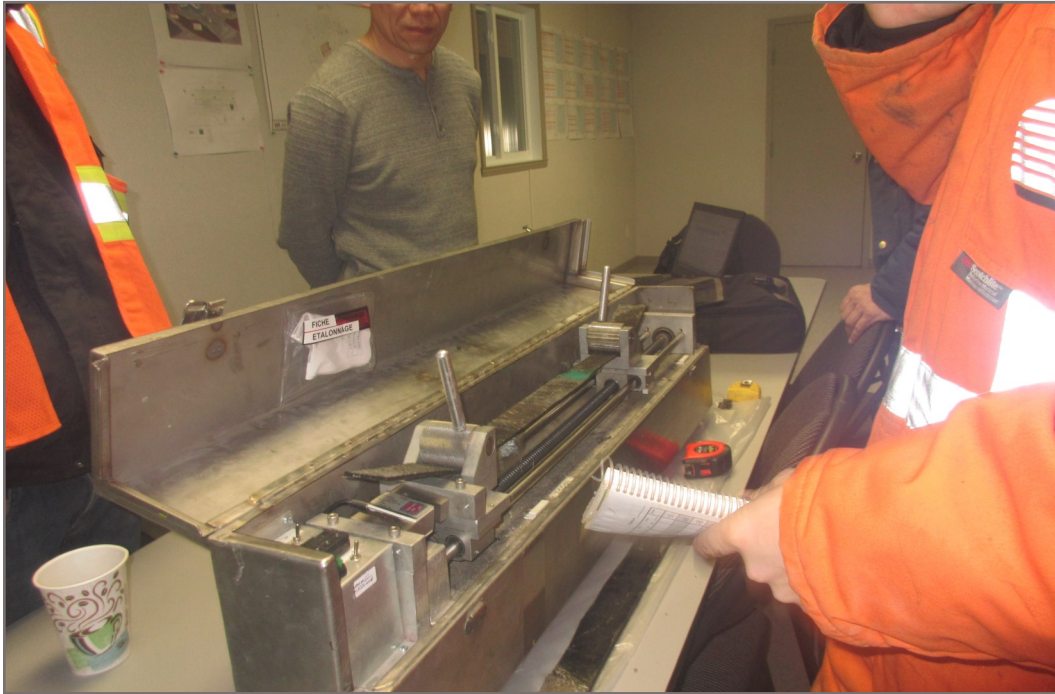
Photo 37: Performing a tensile resistance test on a liner welding pre-qualification test strip
