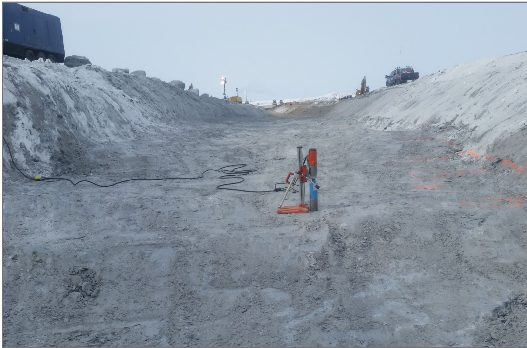
Photo 34: Coring key trench base to take a jar test sample at depth of 2.3 m from OG Station 0+245
