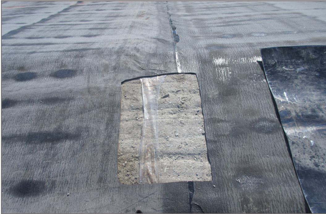
Photo 39: Destructive test sample location between Panels 35 and 36
