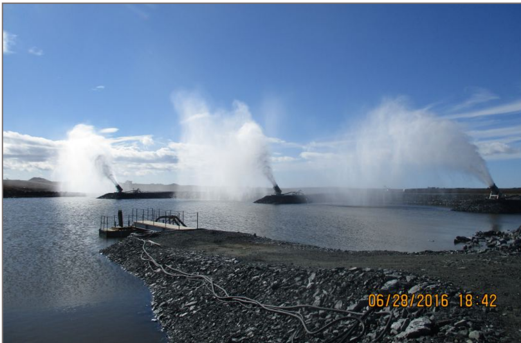
Photo 14: Three evaporators during operation. June 28, 2016.
