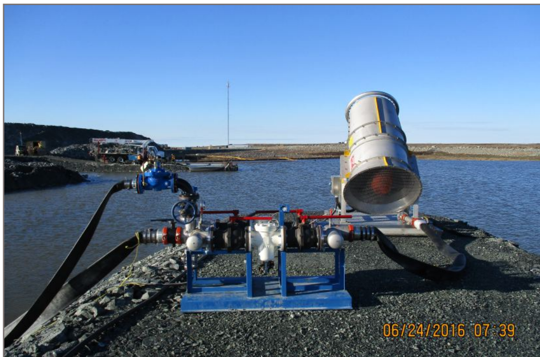
Photo 12: Strainer skid. June 24, 2016.
