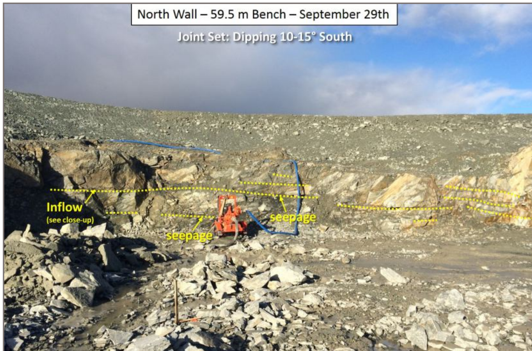
Photo 25: Sub-horizontal jointing associated with water infiltration (looking north)
