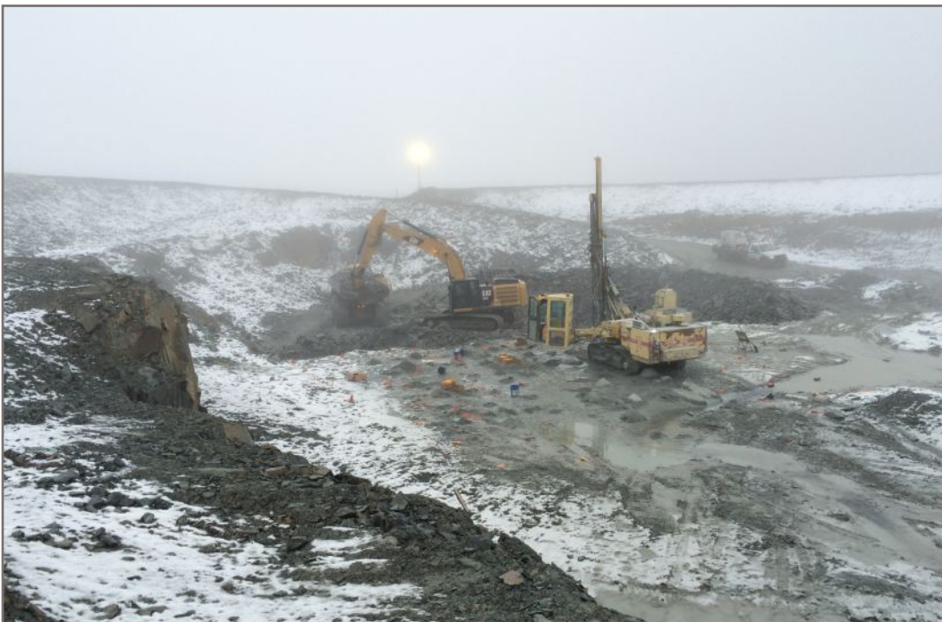
Photo 10: 2.15 m spacing blast pattern (looking east)
