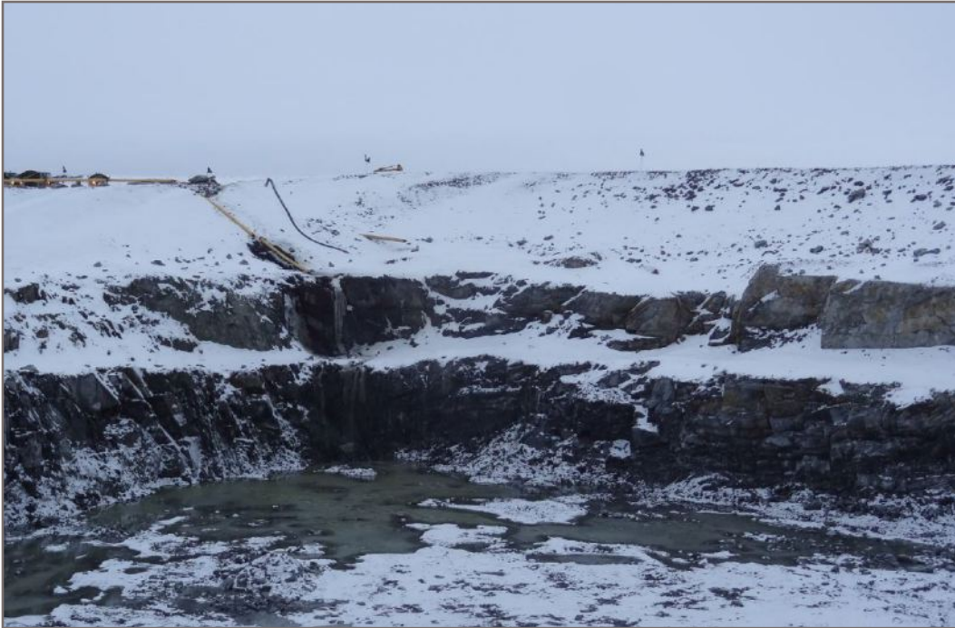
Photo 27: Discharge of saline water onto ROM slope (looking northwest)
