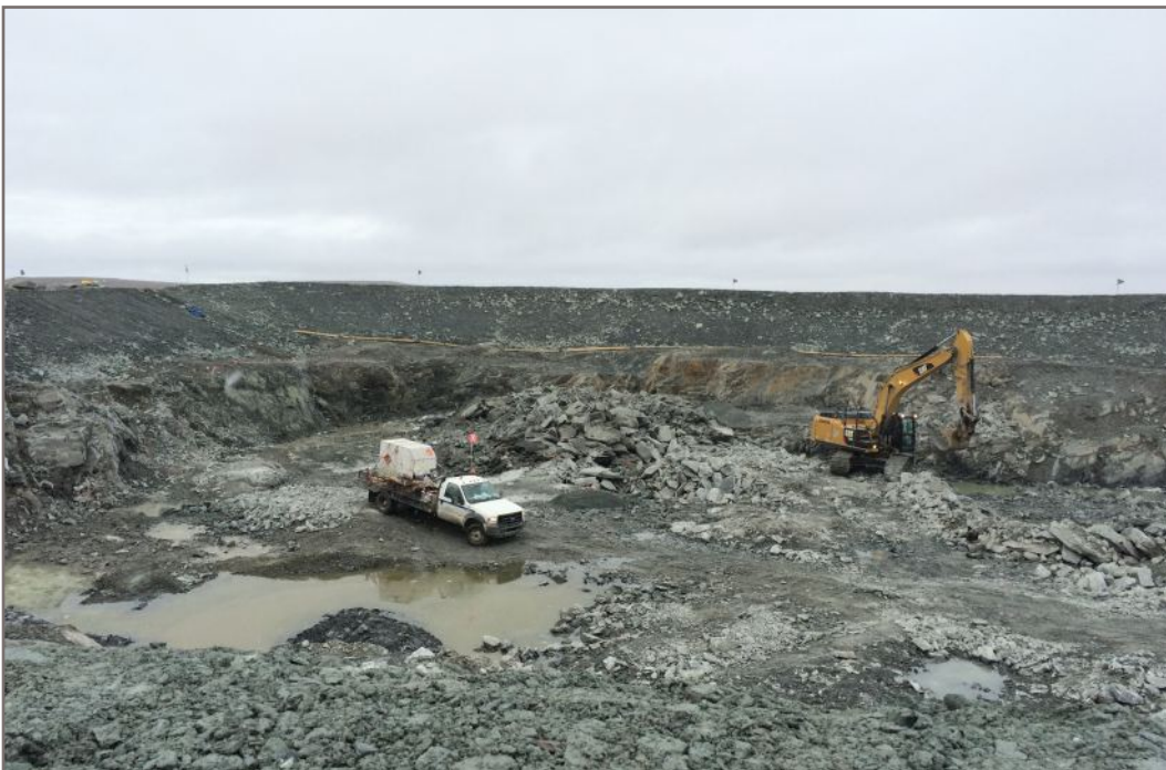
Photo 20: Blast showing oversize material (looking north)
