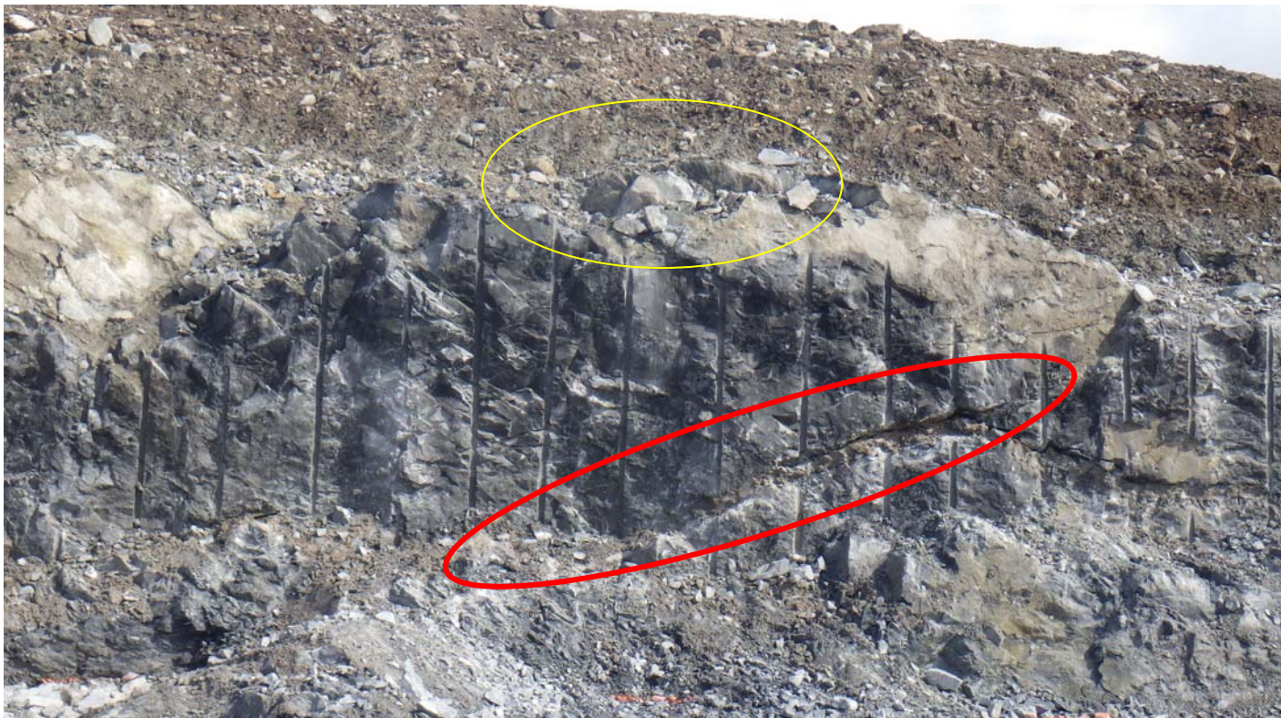
Figure 2 - Inspection area after scaling – showing fault
