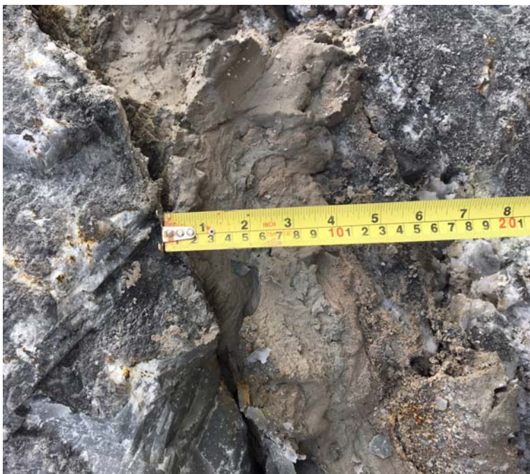
Figure 3 – Fault Gauge – measured thickness (Photo taken by J. Pyliuk, Tetrattech)
