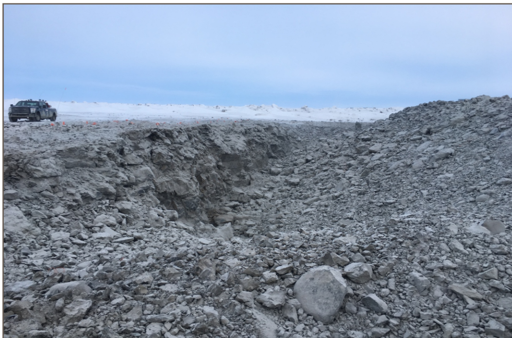
Photo 14: 12 01 2018 Pond CP3 - Rock fragmentation after Blast 4
