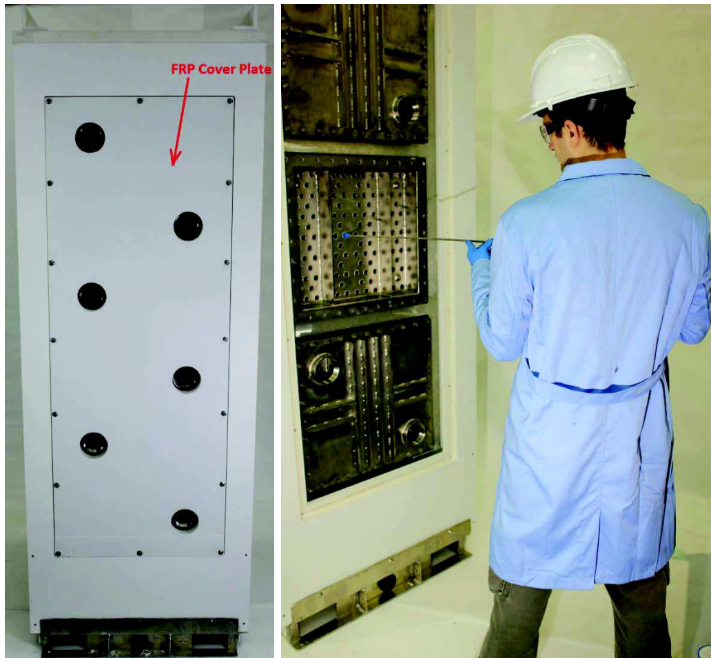
Figure 10: (Left) Heat Recovery Module with external plumbing connections removed. (Right), Radiator module with FRP Cover plate removed and Ti cover plate removed and individual tubes exposed.
