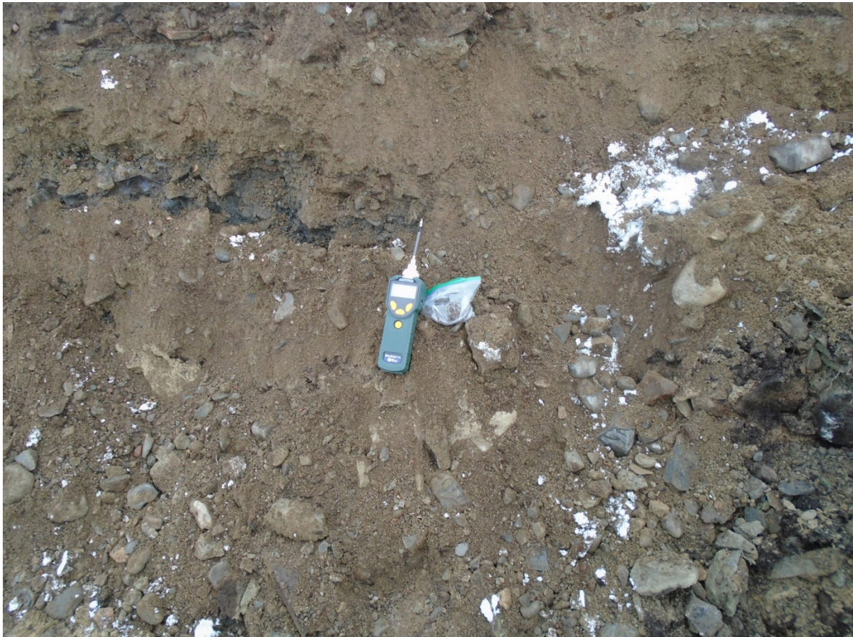
Figure 9 - MiniRAE Lite VOC Gas Monitor
