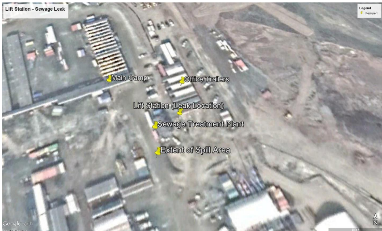
Figure 1: View from above – Main Camp: Location of lift station piping (source of leak) and spill area.
