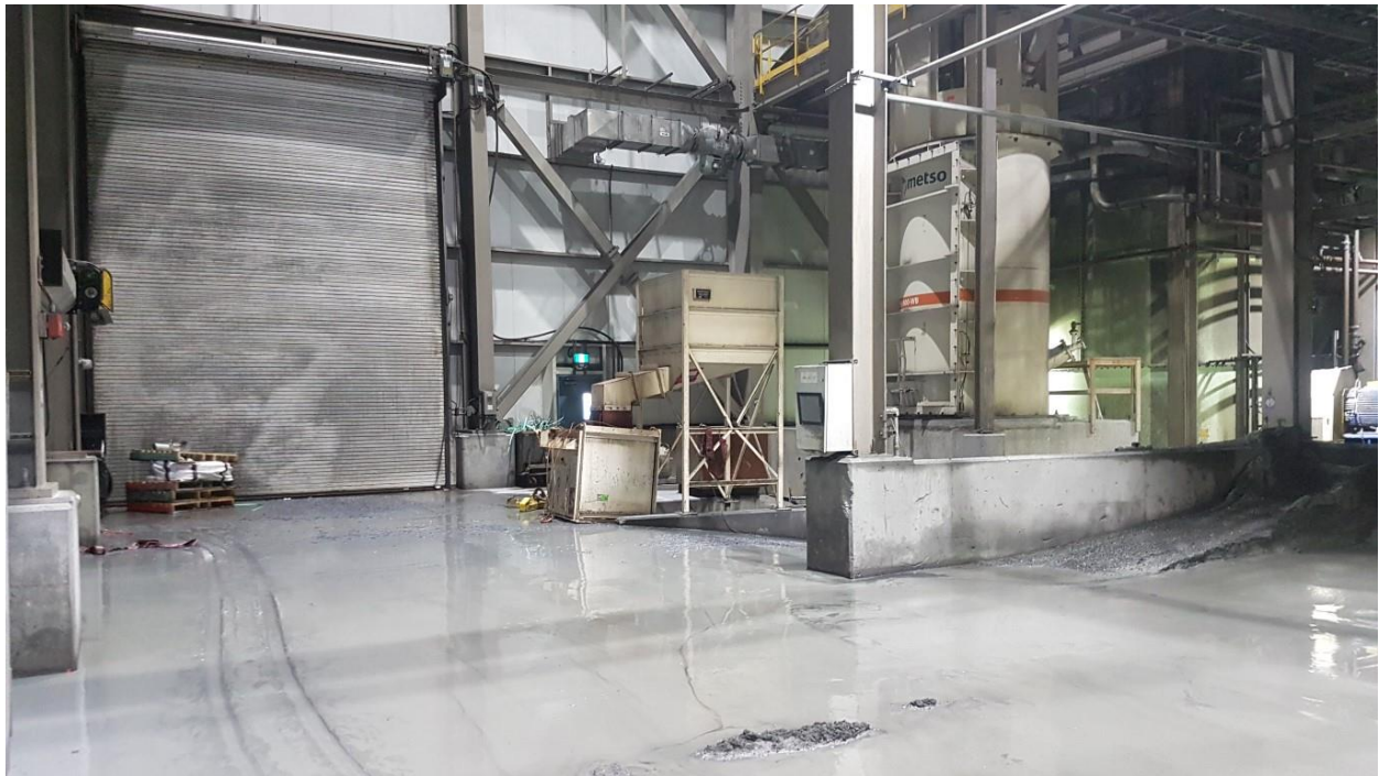
Figure 2: Slurry overflow on Process Plant floor facing south.
