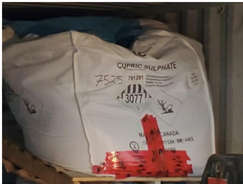
Figure 3: Damaged pallet which has been patched so that no more material is released during transport.
