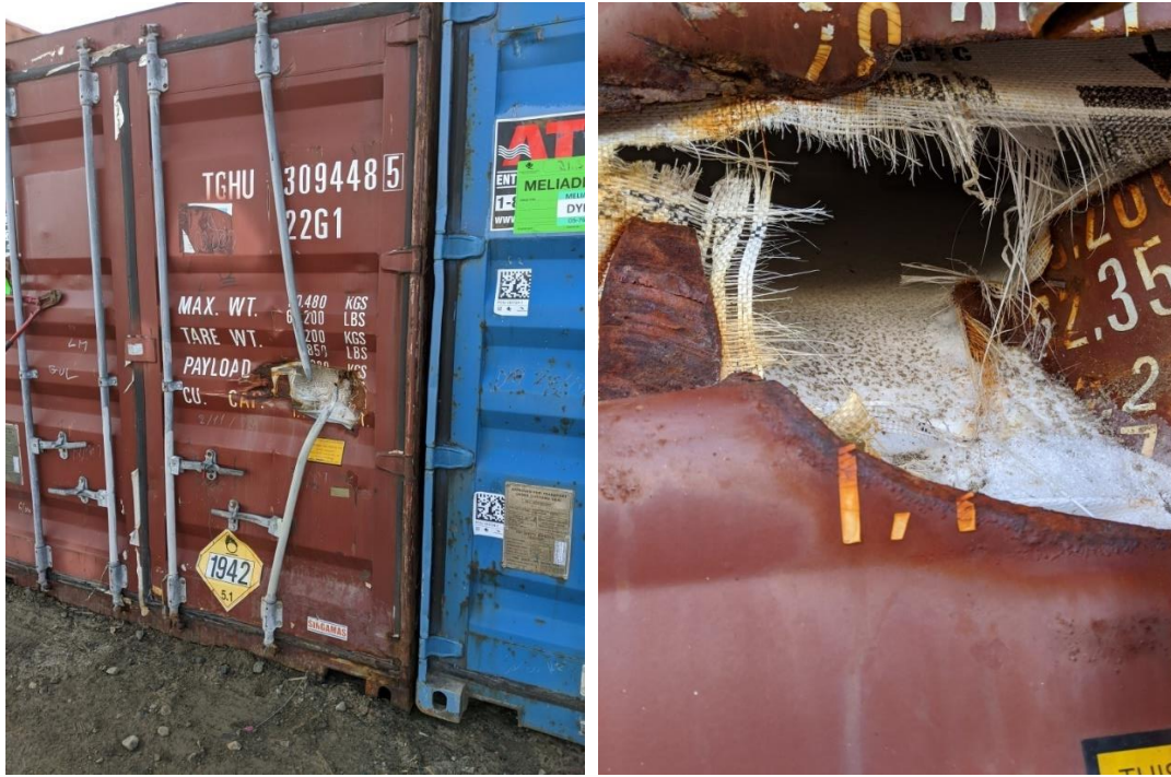
Figure 2: Damaged seacan containing Ammonium Nitrate.
