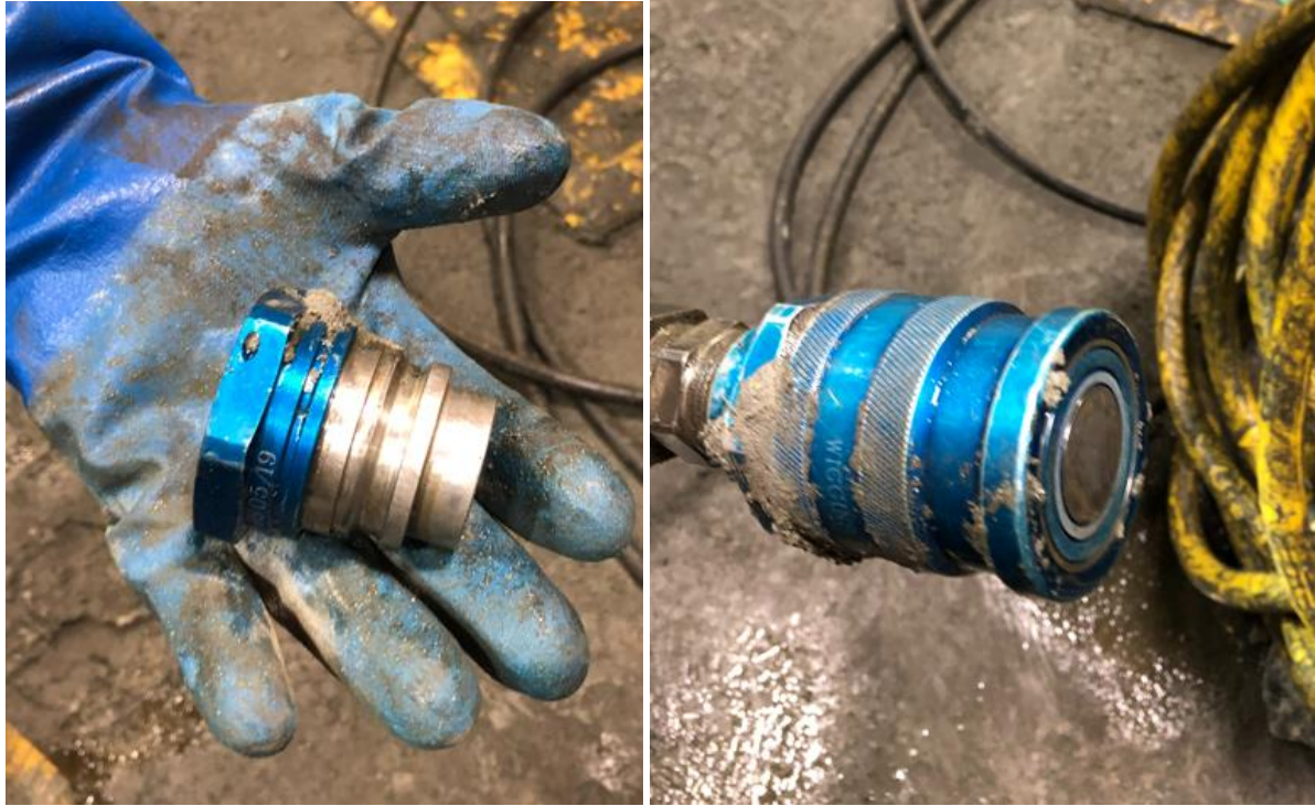
Figure 2: Broken hydraulic line connection from Fuel/Lubrication truck.
