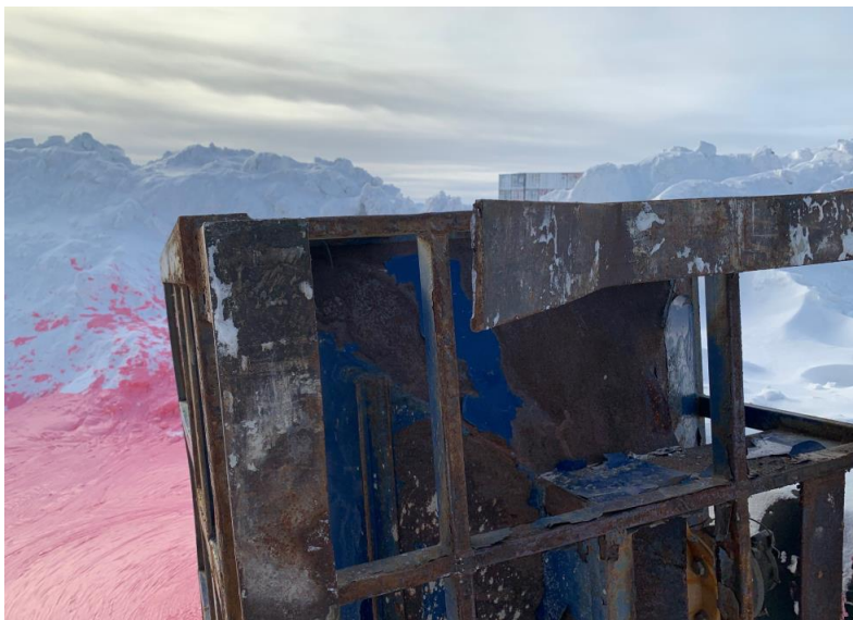
Photo 2: Broken base plate on the bin.
