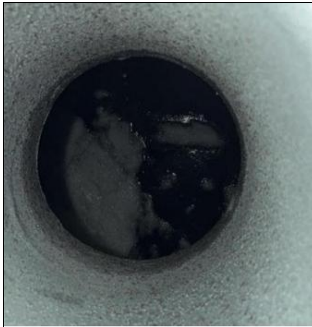
Photo 2: Paraffin in diesel tank from summer fuel being left in tank too late into winter.
