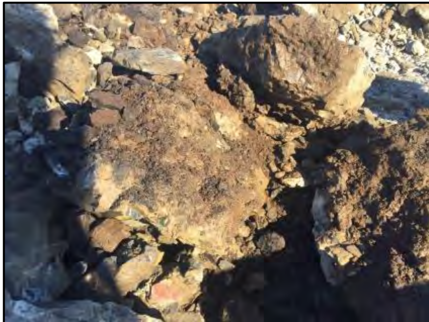
April 15: Free product accumulation at the interface between natural soil and permafrost near field screen location 1.
