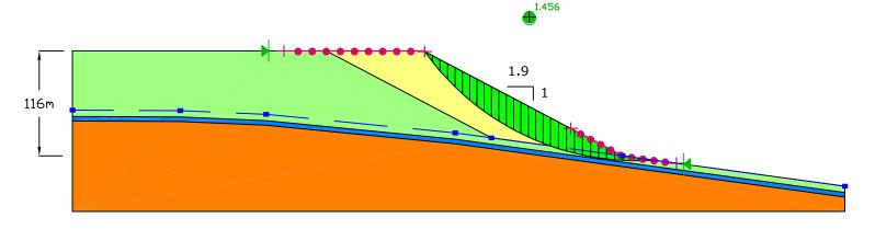
Overburden Failure - No Earthquake Loading - With Water in Overburden
