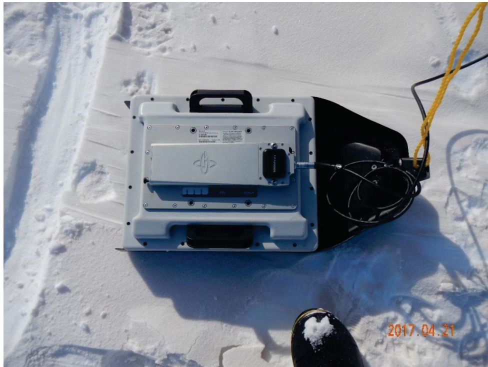
Figure 4: Ground Penetrating Radar Survey Unit
