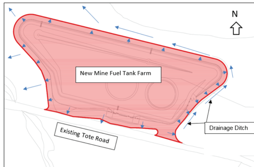
Figure 9-1: New Fuel Tank Farm Drainage
