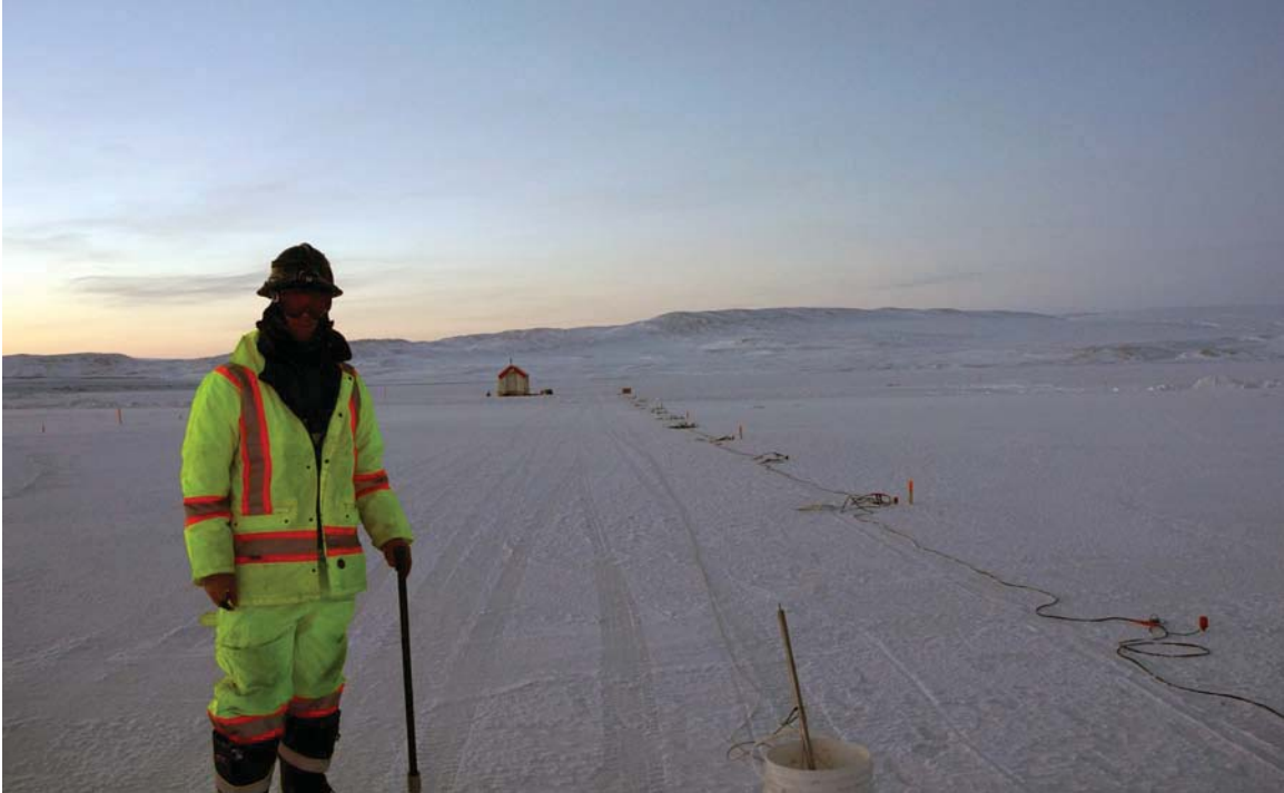
Photo 1: Seismic line setup with buffalo gun
