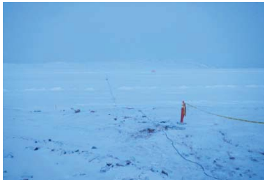
PHOTOGRAPH 6B: Geophone setup
