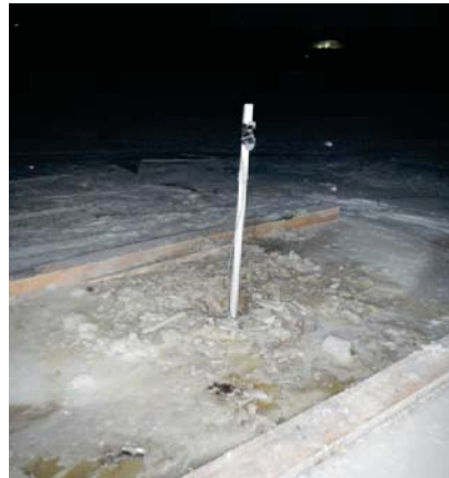
PHOTOGRAPH 4B: PVC pipe with thermistors installed
