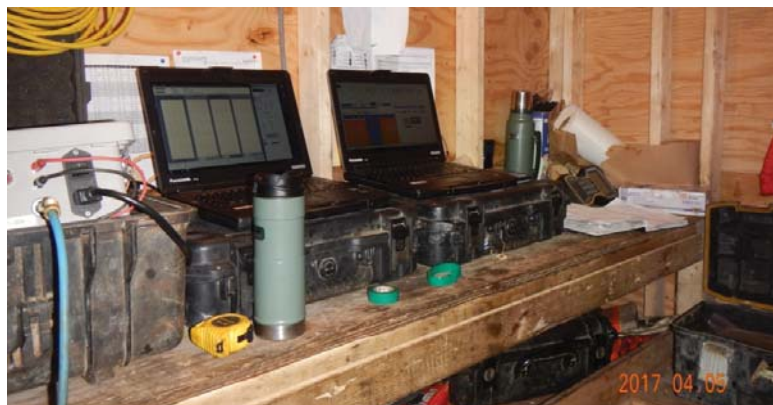
Figure 3: Data Acquisition System for Piezocone Testing
