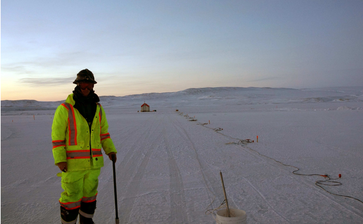
Photo 1: Seismic line setup with buffalo gun
