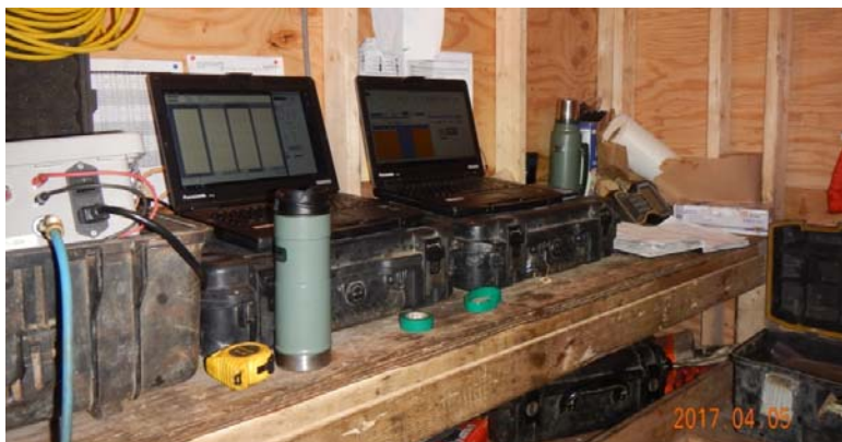
Figure 3: Data Acquisition System for Piezocone Testing
