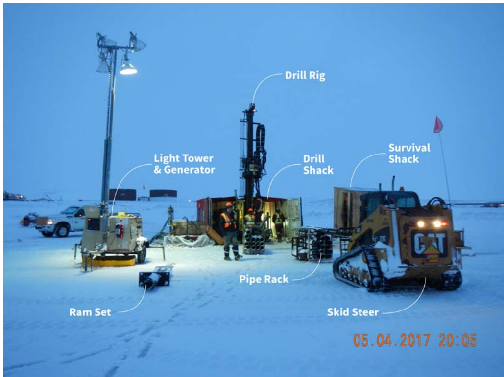
Figure 1: 2017 Offshore Drilling Setup
