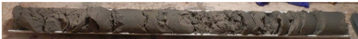
Figure 6: Fine Sand from BH17-D003
