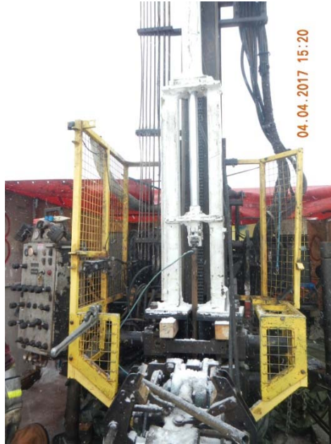
Figure 2: Ramset used for Pushing Cones through the Seabed
