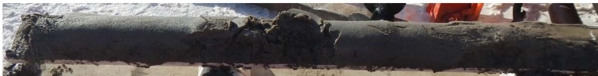
Figure 7: Grey Sand from the Sea Bed, BH17-D001
