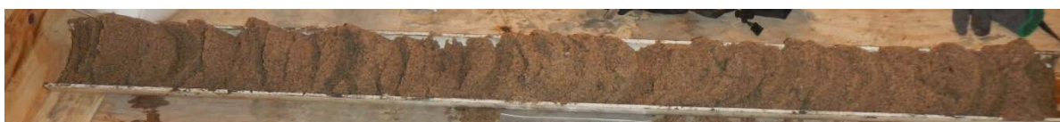
Figure 8: Reddish Brown Sand Encountered in BH17-D001
