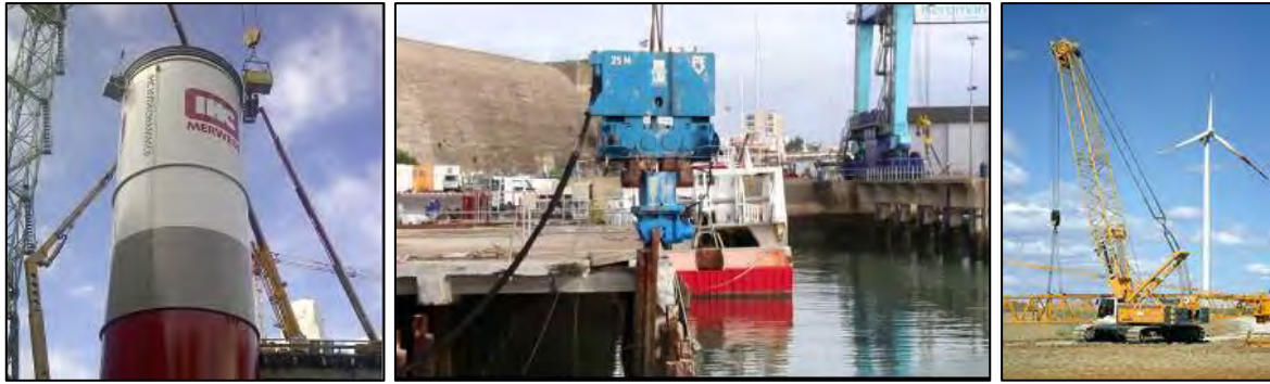
Figure 26 - Hydraulic hammer (left) , Vibro-hammer (middle) & Crawler Crane (right)
