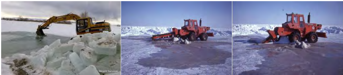
Figure 24: Ice cutting (Ditch Witch) and side casting
