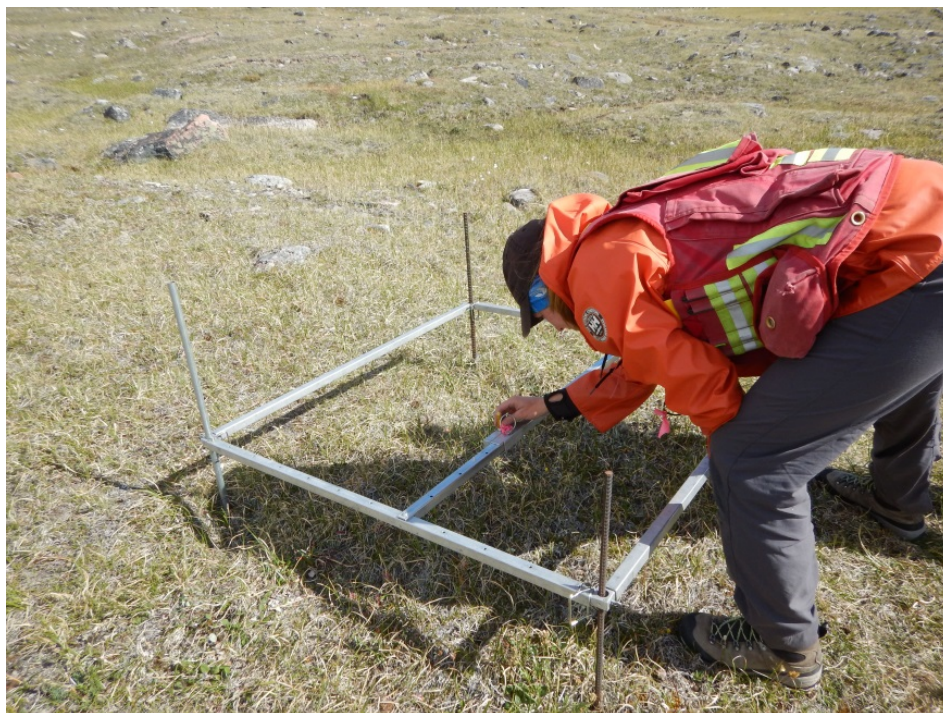
Photo 3. Measuring plot frame erected above the vegetation during sampling, 22 July 2016.
