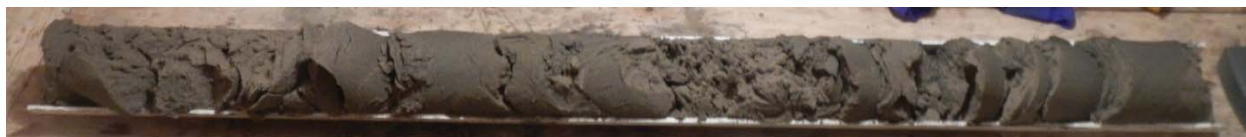
Figure 6: Fine Sand from BH17-D003
