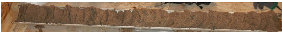
Figure 8: Reddish Brown Sand Encountered in BH17-D001
