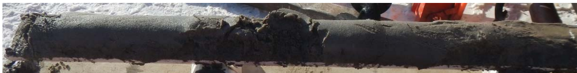
Figure 7: Grey Sand from the Sea Bed, BH17-D001
