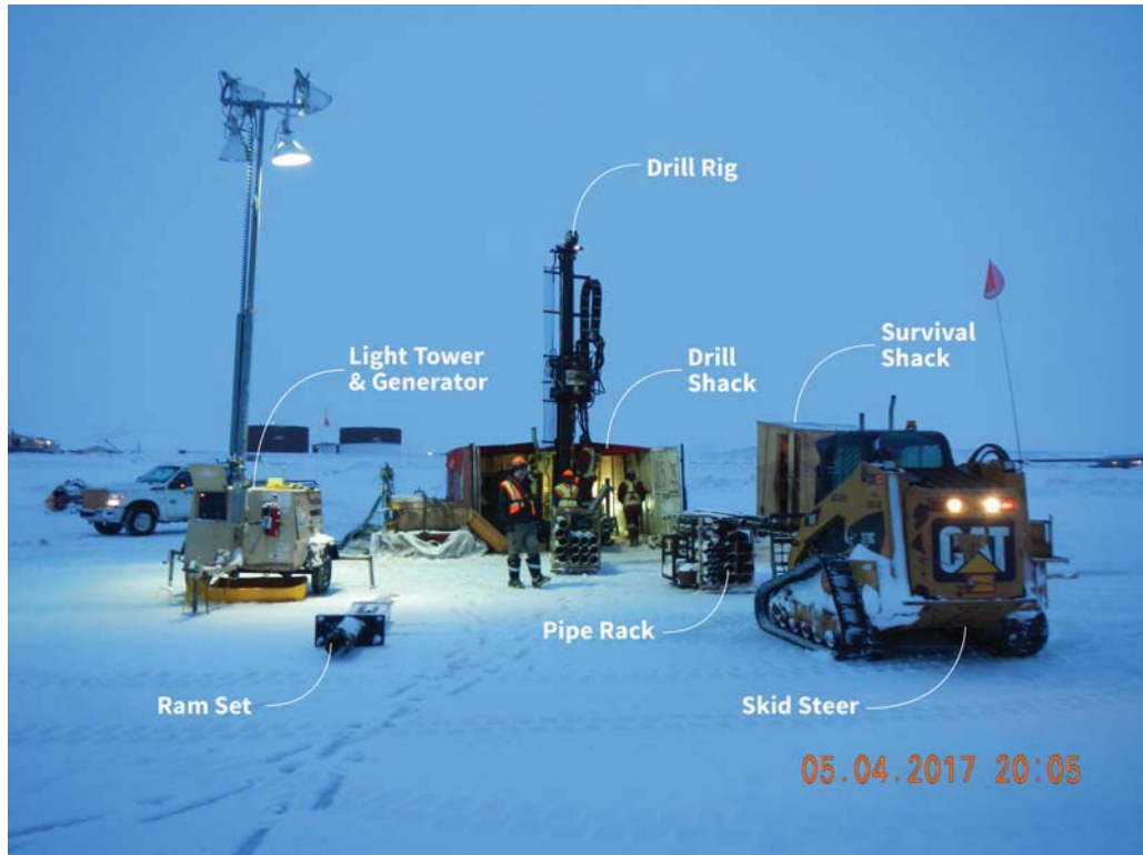
Figure 1: 2017 Offshore Drilling Setup
