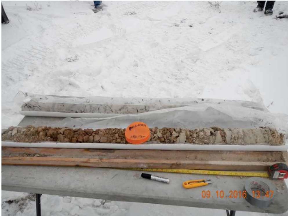
Figure 3: Sample Collected in a PVC Split Using a Mini Sonic Drilling Rig
