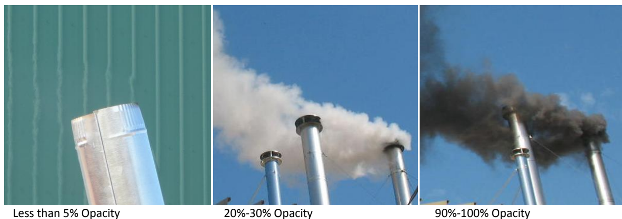
Figure 6 - Examples of Smoke Opacity Ratings
