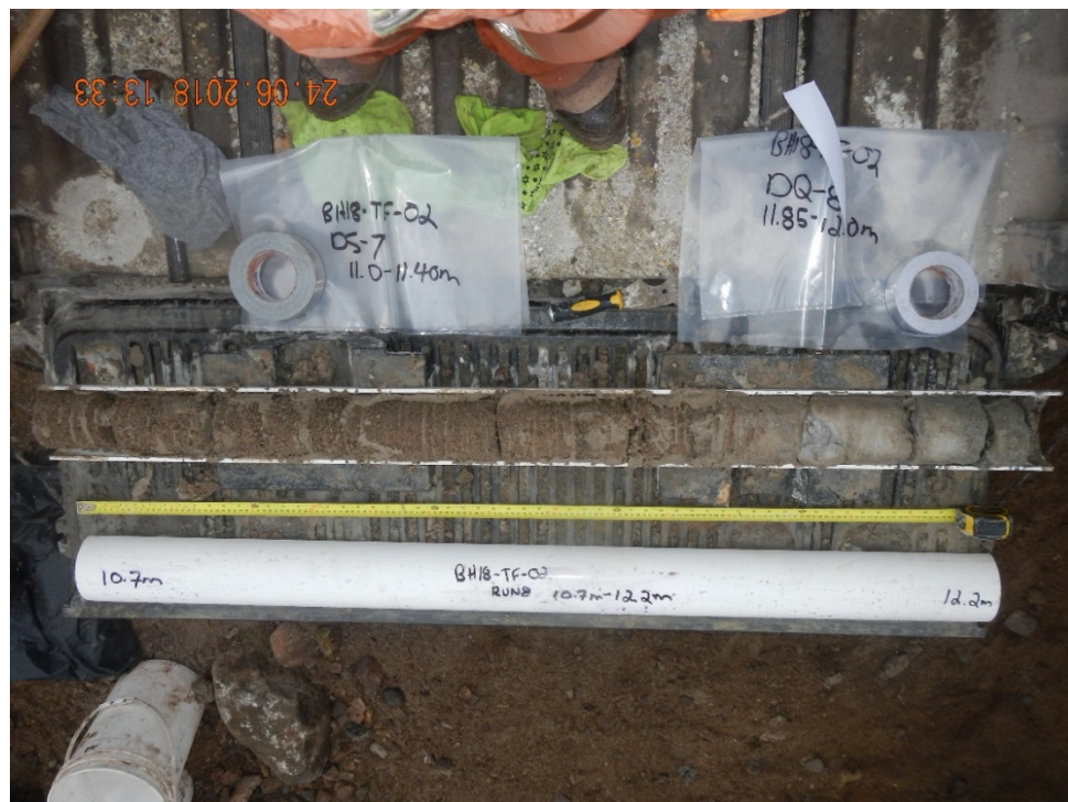
Figure 2-2: Sample Collected in a PVC Split using a Mini Sonic Drilling Rig
