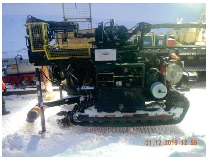
Figure 1: Boart Longyear Mini Sonic Drilling Rig
