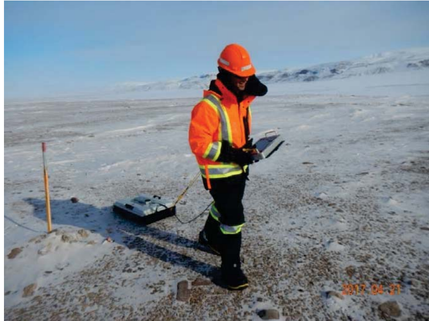
Figure 4: GPR Survey in Progress
