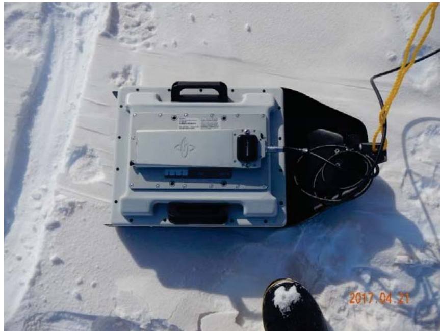
Figure 3: Ground Penetrating Radar Survey Unit
