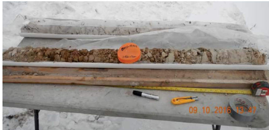
Figure 2: Sample Collected in a PVC Split using a Mini Sonic Drilling Rig
