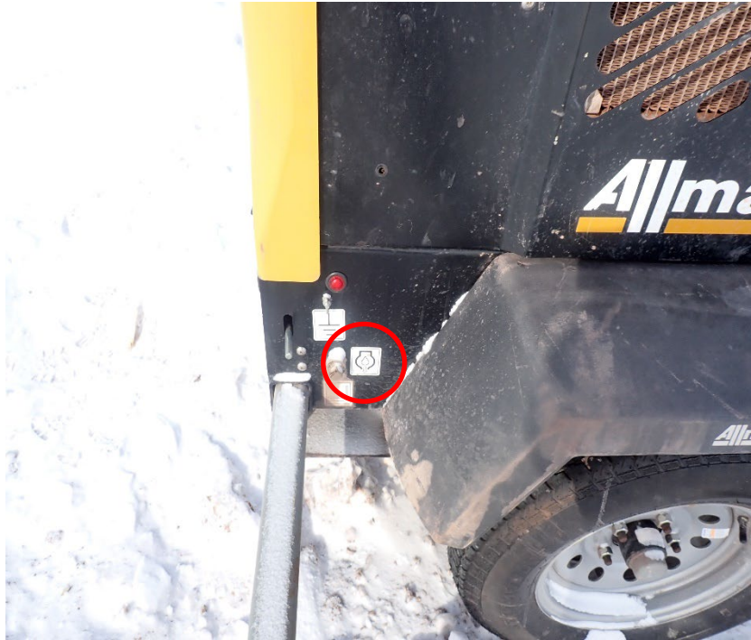
Photo 4: Location of fluid containment system drain plug on the Allmand Night-Lite V-Series located at KM 97, April 20, 2024.
