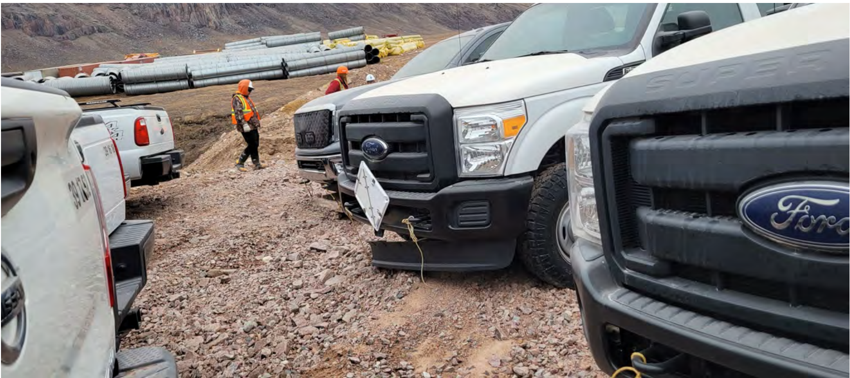
Photo 15A: View of damage starting to happen to parked vehicles at staging area near KM 7 as erosion gully develops beneath them.
