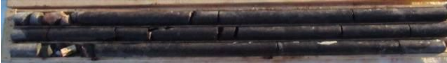
Photo 1: Core Box #1 of 3 (Runs 1-2, 4.2m – 8.3m)
