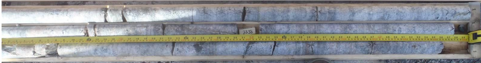
Photo 5: Core Box #6 of 9 (Runs 8-9, 21.1m – 25.4m)
