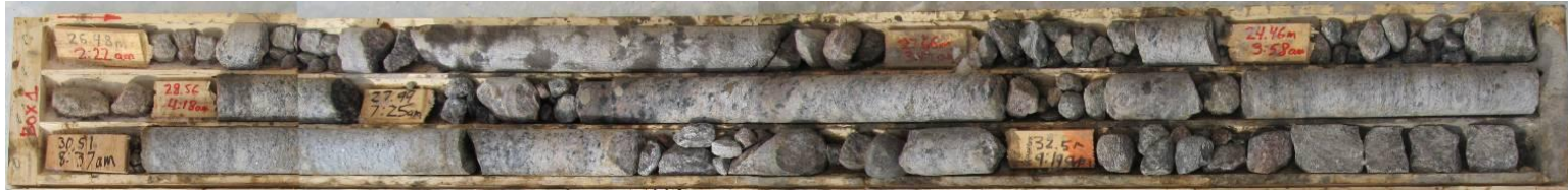
Photo 1: Core Box #1 of 3 (Runs 1-6, 6.6m – 12.4m)
