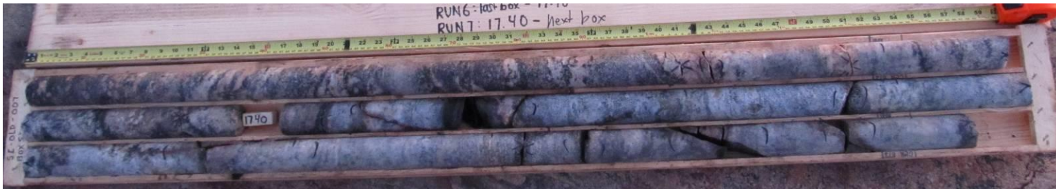
Photo 5: Core Box #5 of 8 (Runs 6-7, 15.6m – 19.8m)
