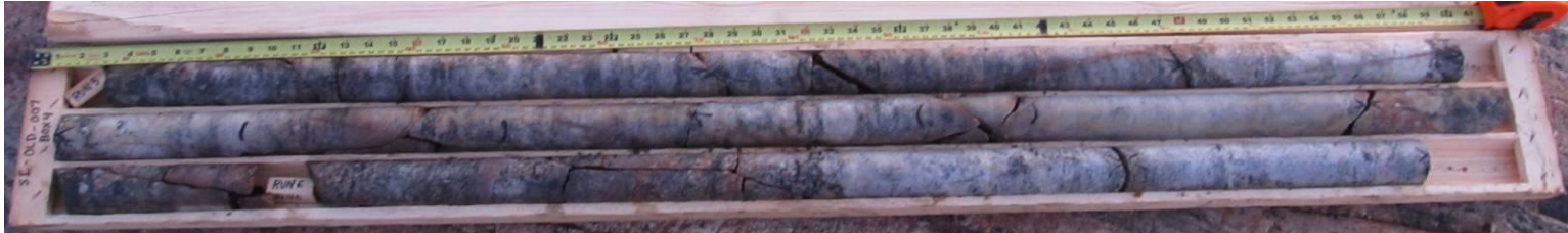
Photo 4: Core Box #4 of 8 (Runs 5-6, 11.4m – 15.6m)
