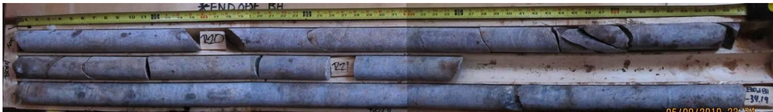
Photo 4: Core Box #4 of 4 (Runs RC-18 to RC-20, 24.6m – 27.9m)
