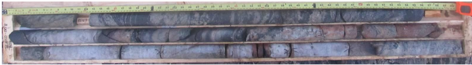
Photo 2: Core Box #2 of 9 (Runs 2-4, 4.2m – 8.5m)
