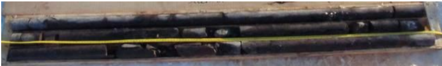
Photo 2: Core Box #2 of 3 (Runs 2-3, 8.3m – 12.8m)
