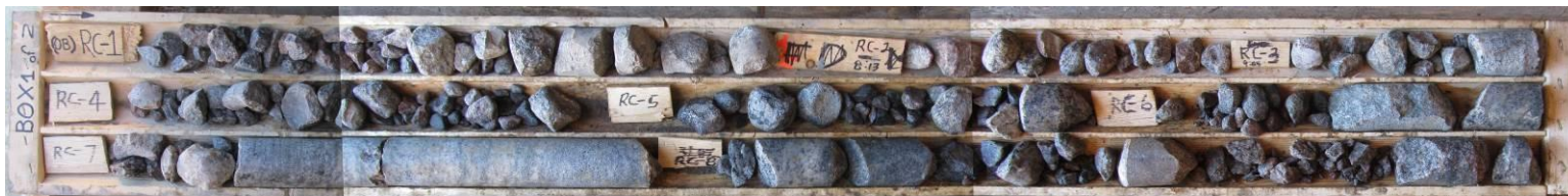
Photo 1: Core Box #1 of 2 (Runs RC-1 to RC-8, 11.2m – 20.6m)
