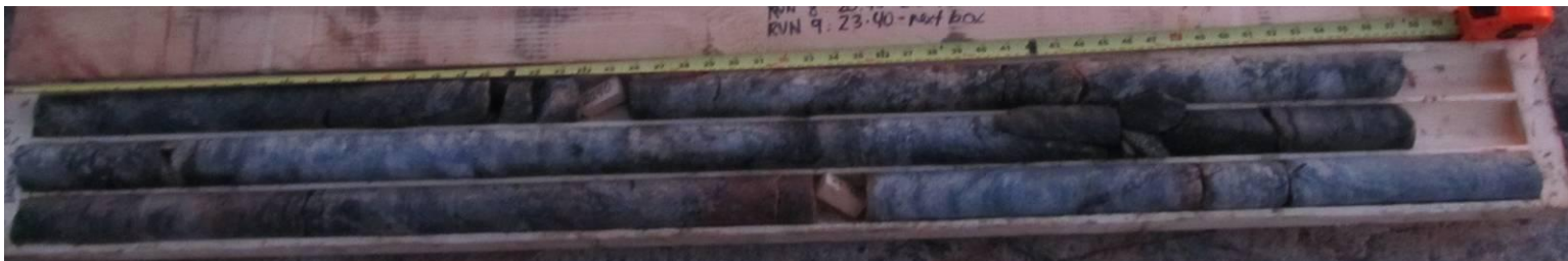
Photo 6: Core Box #6 of 8 (Runs 7-9, 19.8m – 24.0m)
