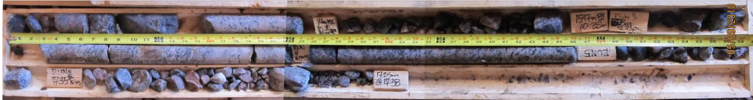
Photo 1: Core Box #1 of 4 (Runs RC-2 to RC-6, 7.0m – 11.0m)
