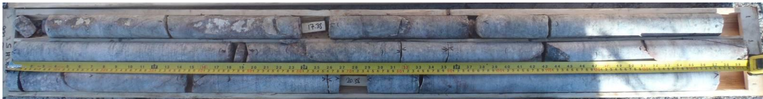
Photo 4: Core Box #5 of 9 (Runs 6-8, 16.9m – 21.1m)
