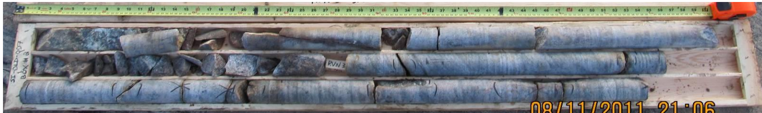
Photo 2: Core Box #2 of 8 (Runs 2-3, 3.9m – 7.3m)
