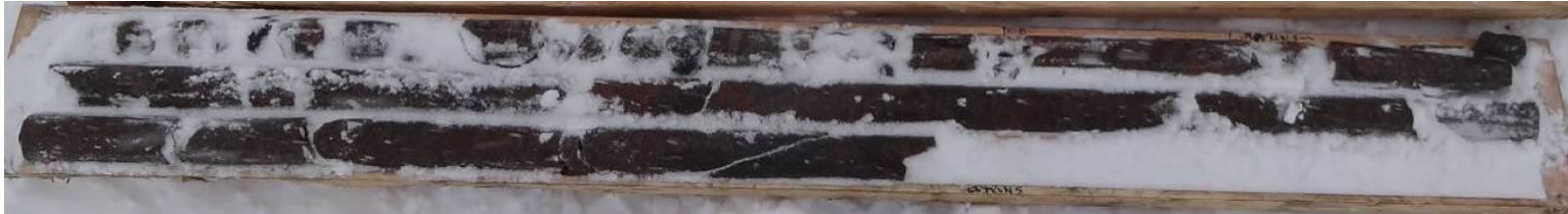
Photo 1: Core Box #1 of 3 (Runs 1-5, 0.0m – 15.2m)
