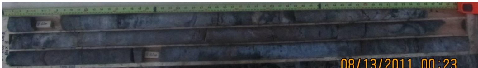
Photo 3: Core Box #3 of 9 (Runs 4-6, 8.5m – 12.6m)
