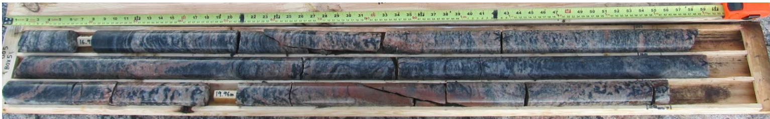
Photo 5: Core Box #5 of 8 (Runs 6-8, 16.9m – 20.8m)
