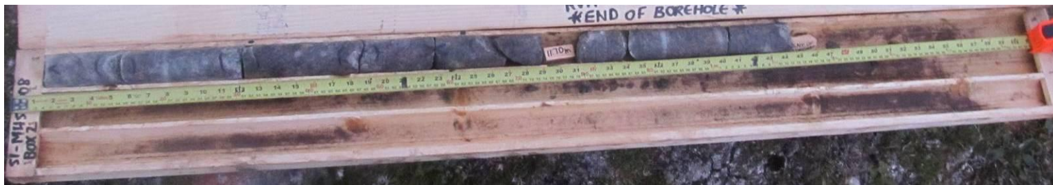
Photo 2: Core Box #2 of 2 (Runs 4-5, 11.0m – 14.7m)
