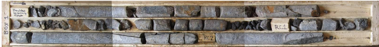
Photo 1: Core Box #1 of 2 (Runs 1-2, 0.0m – 12.3m)
