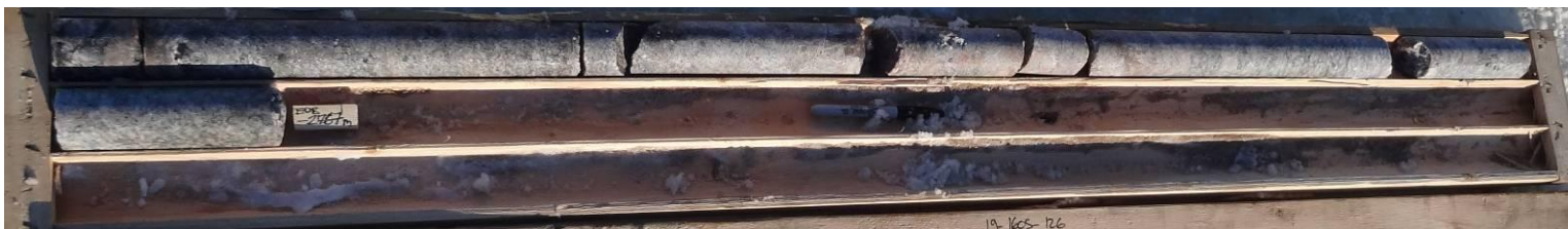
Photo 3: Core Box #3 of 3 (Run 5, 16.0m – 17.7m)
