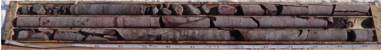
Photo 1: Core Box #1 of 2 (Runs 1-3, 0.0m – 11.3m)
