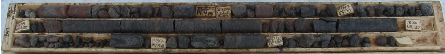
Photo 1: Core Box #1 of 4 (Runs 1-5, 5.0m – 14.2m)
