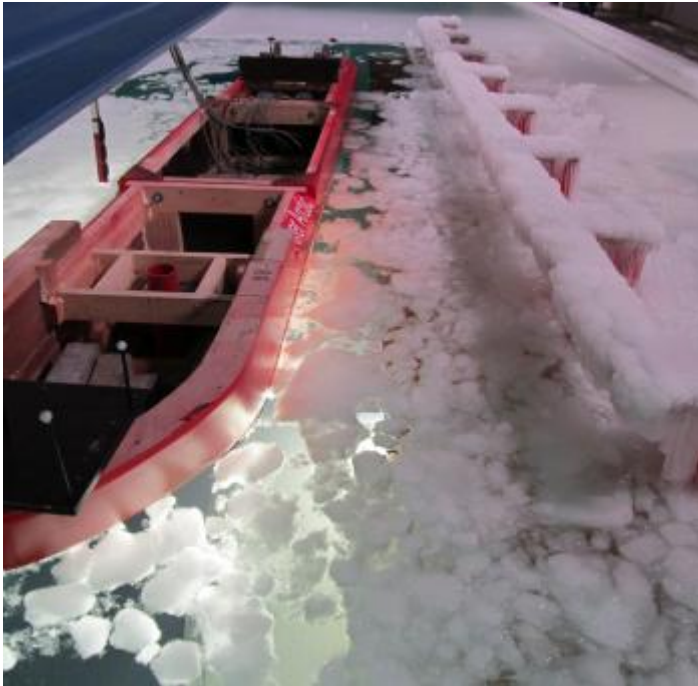
Figure 5-18: The managed ice in front of the dock before the vessel was pushed to the dock.
