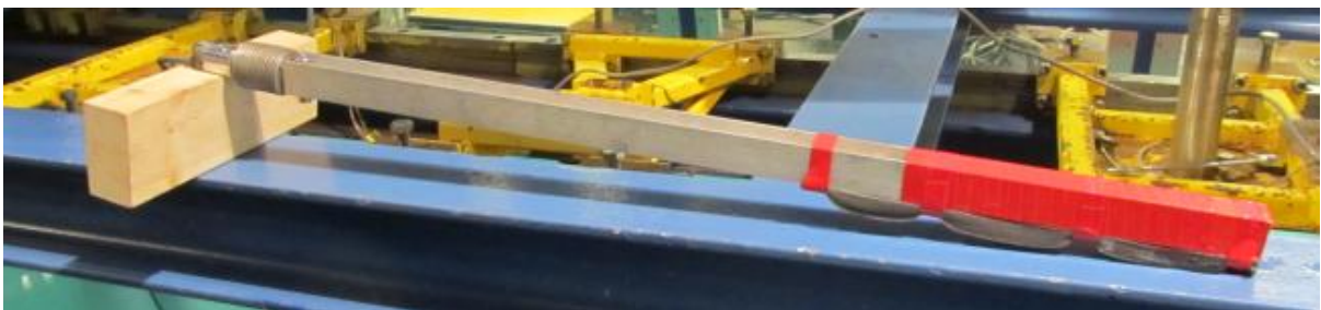
Figure 4-5: Shear force transducers were installed onto the upper end of the shafts.
