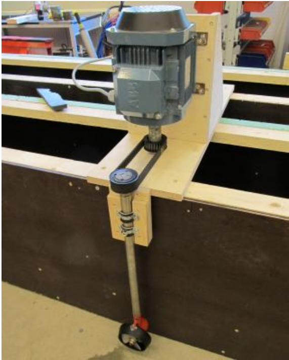
Figure 4-4: A small thruster was installed onto the bow of model in order to simulate a harbour tug pushing the vessel.
