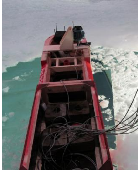
Figure 4-4: A small thruster was installed onto the bow of model in order to simulate a harbour tug pushing the vessel.
