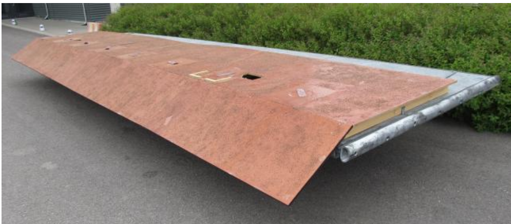
Figure 3-5: The artificial bottom on which the terminals were mounted.
