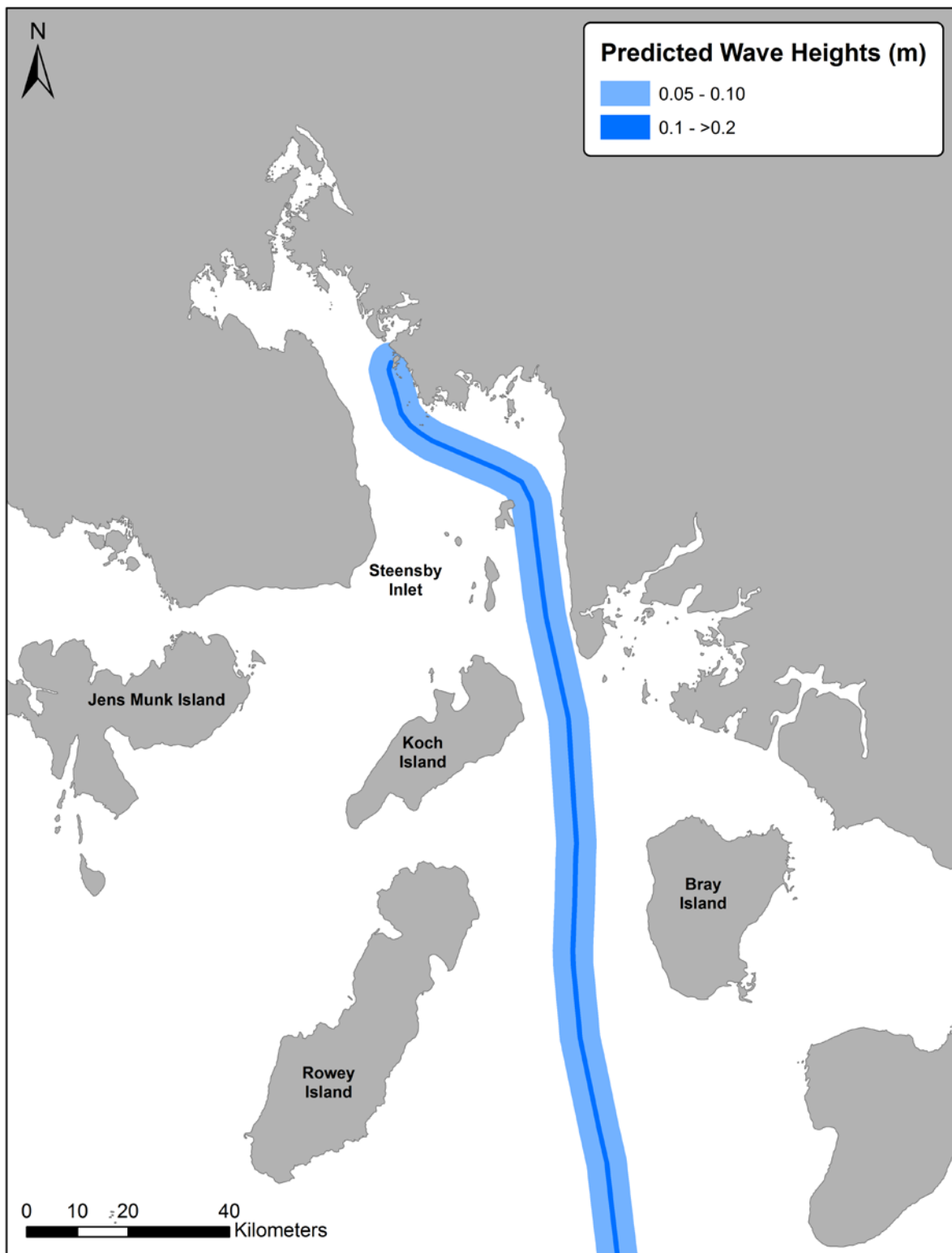
Figure 2. Wake heights resulting from a 14 knot ship transit speed (after Kreibel 2003 and Appendix 8D-1 Figures 8D-1.1 – 8D-1.4).
