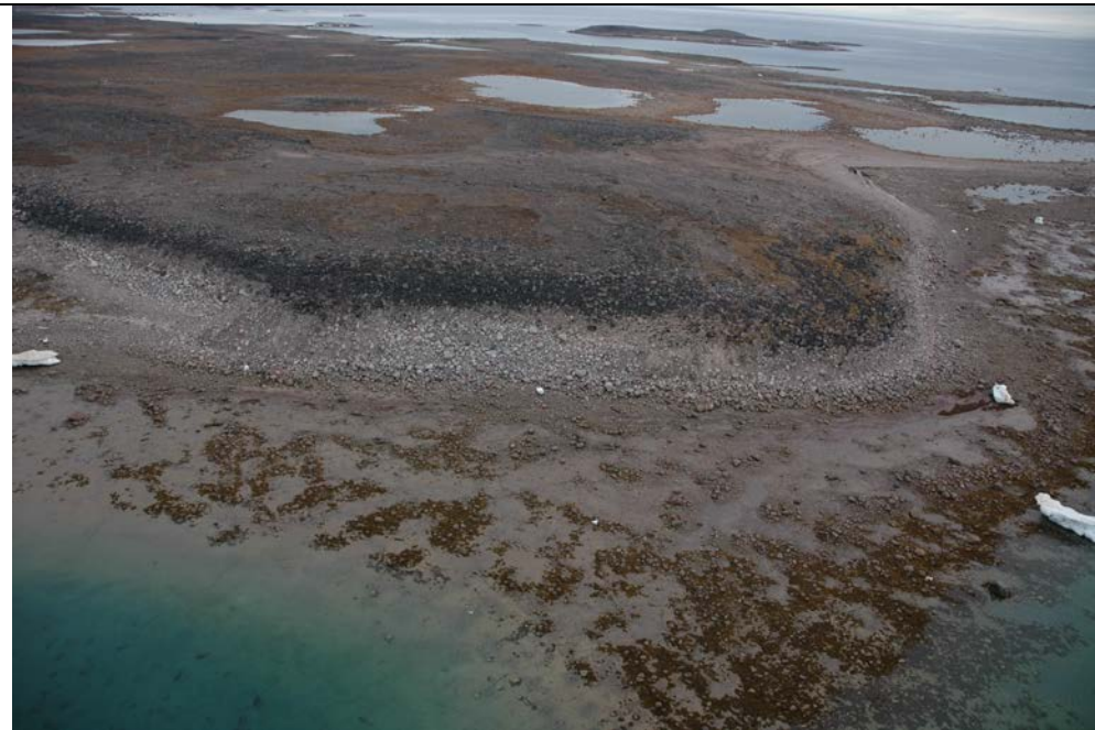
Figure 7. Aerial photo of typical shoreline immediately south of the proposed port area (Location B, Fig. 3). the upper intertidal zone is boulder and the lower intertidal zone is a mixture of boulder to sand-sized sediment. Rockweed ( fucus ) covers the boulders in the lower intertidal. While some intertidal sands exist, the boulder cover 40-50% cover) is likely to anchor the shoreline from any significant erosion. Raised beaches in the backshore indicate the shore is isostatically rising.
