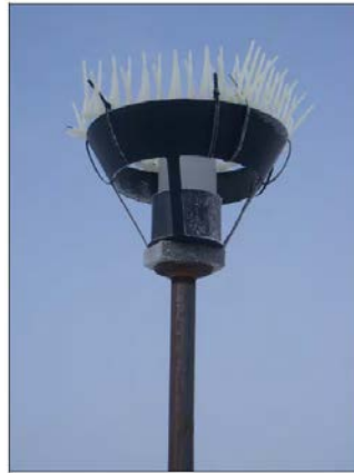
Photo 1. Dustfall collector sampling apparatus (from Rescan 2012).
