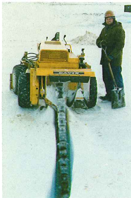
Davis tractor, fitted with chainsaw-type ice cutter, simplified first step of cutting doughnut-shaped trench; crane clammed out 5 ft cubes of ice.
