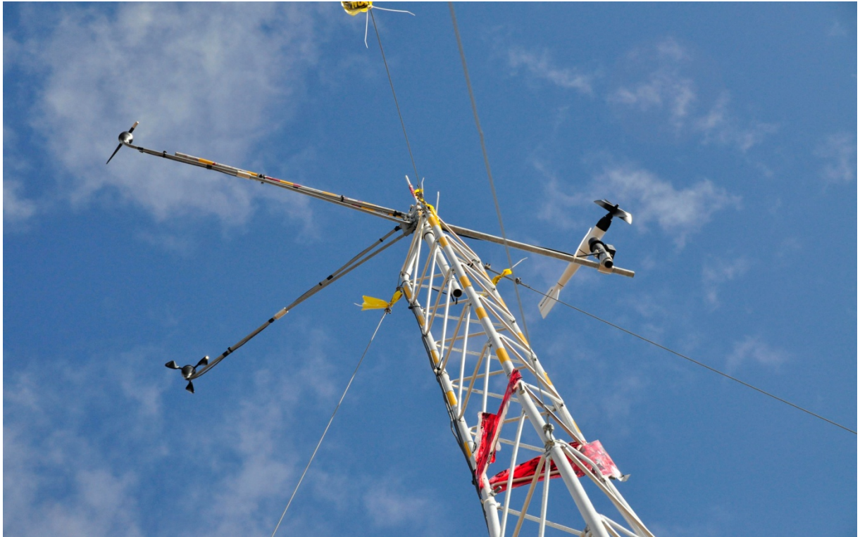
Photo 1: Campbell Scientific Weather Station – Top of 10-m tower
